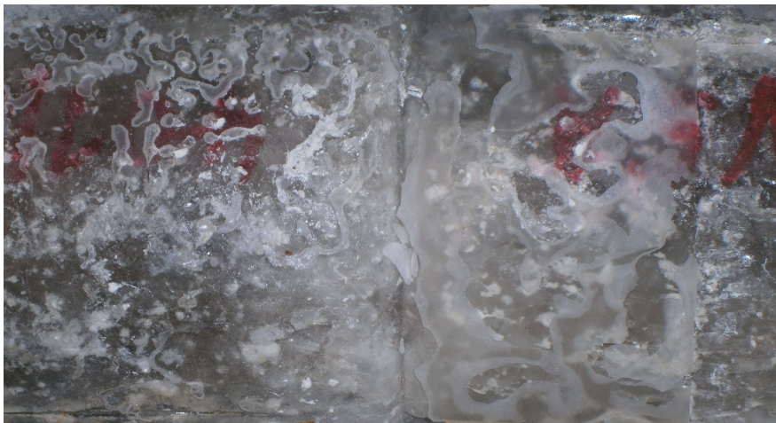
Fig. 3. Rock salt cores with polymerized sodium silicates. The specimen was stored about three months in an air-tight plastic tube at room temperature.
