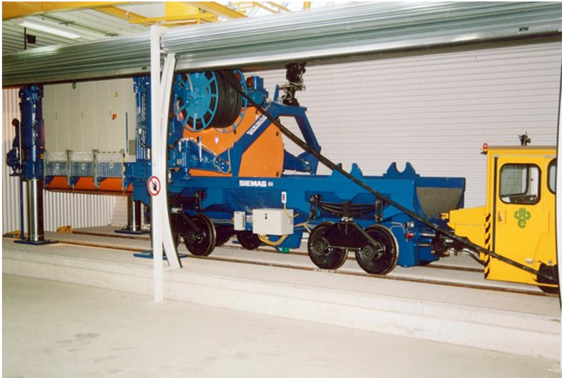
Fig. 2. Demonstration facility with emplacement device and transport cart
