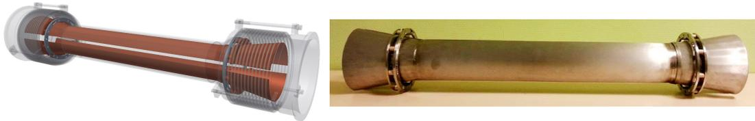
Figure 3.8.: DPS electric dipole system. The dipoles are placed inside the DPS beam tube module two, three, and four. Left: CAD model inside one beam tube element. Right: Dipole prototype.
