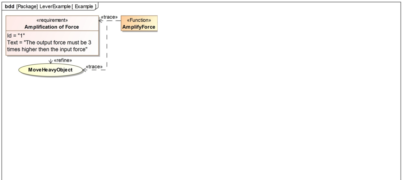
Fig. 1. State 1 of the model: At the beginning of FES a {«Function» AmplifyForce} and further information is given
