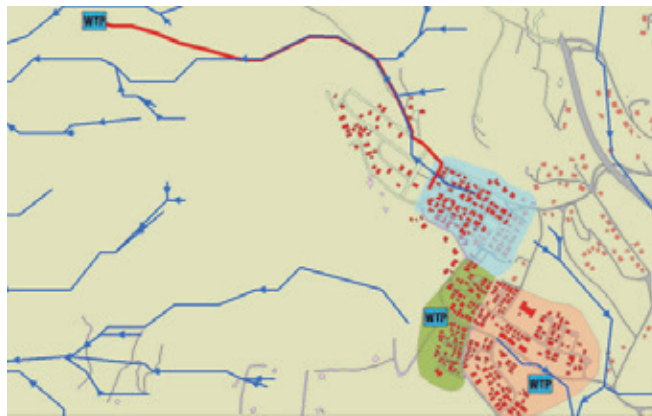
Figure 66: Decentralized wastewater treatment scenario for Maghareeb.
