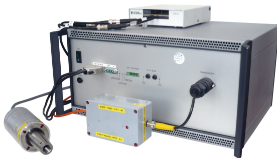
(a) Amplifier TIB S250K, transformer and converter TIB HS USW 1000 with customised National Instruments I/O connector block SCB-68
