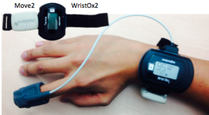
Figure 6.11: Sensor data collection platform for pre-triage study
