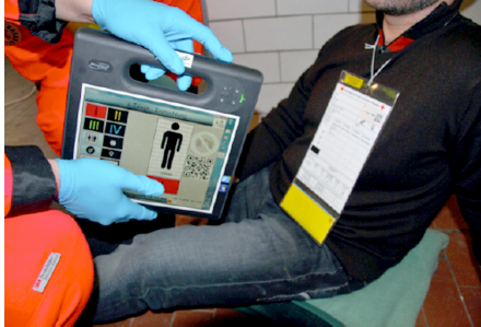
Figure 3.7: Triage tag with RFID from e-Triage project [DEA + 11]
