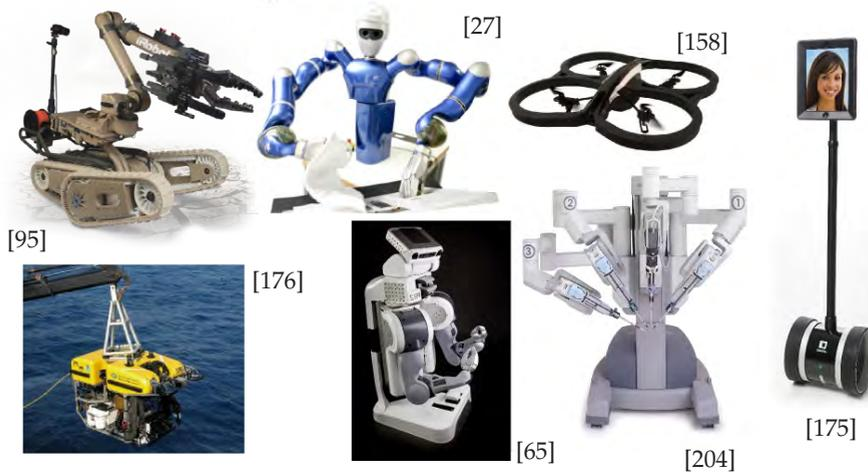
Figure 2.3.: Some examples for remote robots in the fields of minimal invasive surgery [204], inspection [158], deep sea [176], or military intervention [95], general-purposed robots [27, 65], and telepresence robots used as advanced video conferencing tools [175].
