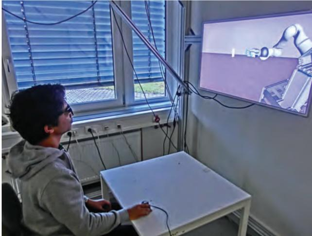
Figure 5.13.: Setup for Study 3 to evaluate the assistance for hand positioning with virtual fixtures.
