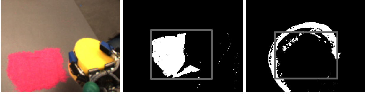
Figure C.2.: Left: Robot view from the scene. Center: Segmented view of the scene in the beginning of the wiping execution. Right: Segmented view on a "clean" table.
