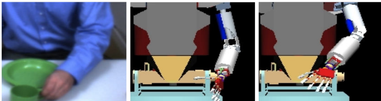
Figure 8.13.: Left: View on the arm configuration observed using the upper body tracking method. Center: Reproduction of the captured arm configuration. Right: Depiction of the optimized joint angle configuration using the MMM interface.
