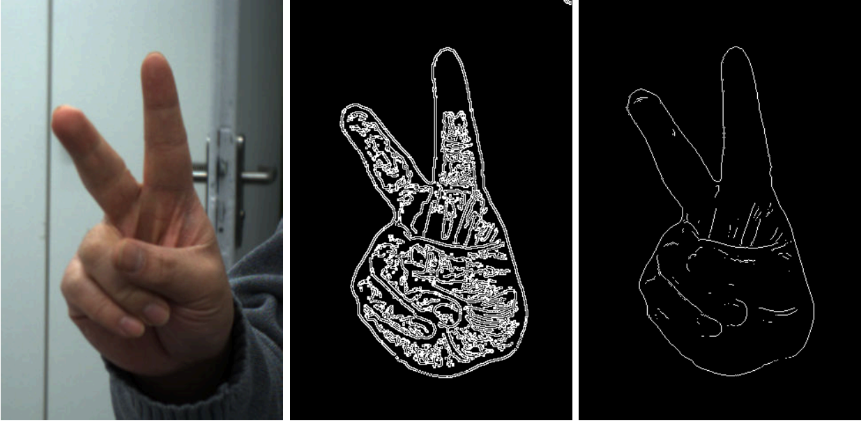
Figure 5.5.: Left: Original input image. Center: Edge image using Canny detector. Right: Edge image using the method proposed in Section 5.3.5.
