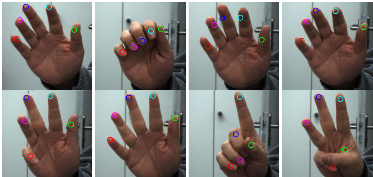
Figure 8.2.: Images of the tracking results. The upper row depicts simultaneous closing of the fingers, while the lower row shows sequential flexing of the fingers. The fingertips are labeled as follows: Thumb (green), index (light blue), middle (dark blue), ring (pink), and pinkie (red).
