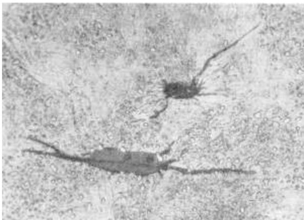
fig. 2.1.: Crack initiation at NMIs as published in [LP47]
