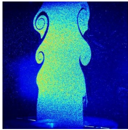
Figure 3.3: The Kelvin-Helmholtz shear layer rollup in a round jet, LIF cross section. Reproduced from [116].
