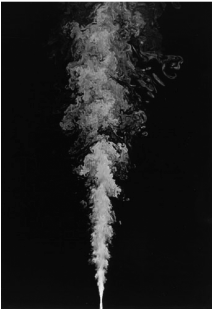
Figure 4.1: Liquid-phase turbulent jet symmetry plane slice. Gray scale codes jet-fluid mole fraction. Reynolds number approximately 10^4 . Reproduced from [22].
