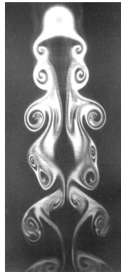
Figure 3.8: LIF visualization obtained by placing the laser sheet parallel and very close to the wall ( x/D = 0.2 , R = 2 ). Reproduced from [13].
