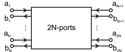
(b) 2 \times N port power wave (a, b) definition
