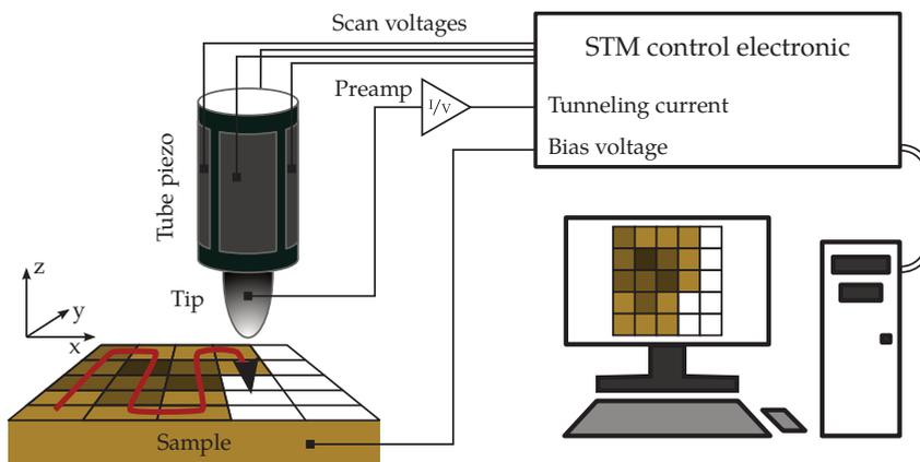
**Figure 2.6:** Basic principle of an STM. The metallic tip is moved in a grid over the scan area by the use of a piezo-tube. A bias voltage is applied to the sample, which yields a tunneling current flowing from the sample to the tip. This current is amplified by a preamplifier and measured in a control electronic. At every pixel the tunneling current, the position of the tip etc., are recorded by a computer. Thereby, a false color image is produced.
