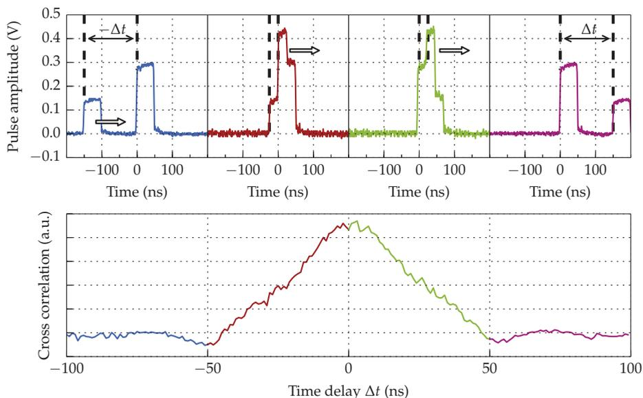
**Figure 4.7:** Test measurement using the 9530 digital delay pulse generator. In the upper row different situations of the real time pulse shapes are shown. A pump pulse of 0.3 V and a probe pulse of 0.15 V were generated. Both are 50 ns wide. They were measured using an oscilloscope. The spectrum in the lower row shows the cross correlation of the pulses in an STM tunneling junction. Therefore, the delay time  $\Delta t$  was varied. A W-tip and a nonmagnetic Ir sample were used.
