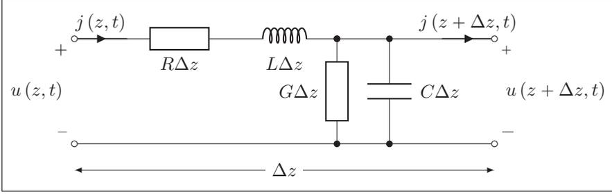
**Figure 4.3:** Lumped-element representation of an infinitesimal part  $\Delta z$  of a microwave transmission line.  $R$  (resistance in series),  $L$  (inductance in series),  $G$  (shunt conductance) and  $C$  (shunt capacitance) are per-unit-length quantities. The characteristics of voltage  $u(z, t)$  and current  $j(z, t)$  over the transmission line are the quantities of interest.
