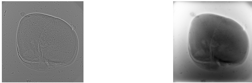
(a) Enhanced edges in a phase contrast image. (b) After phase retrieval and correction.
