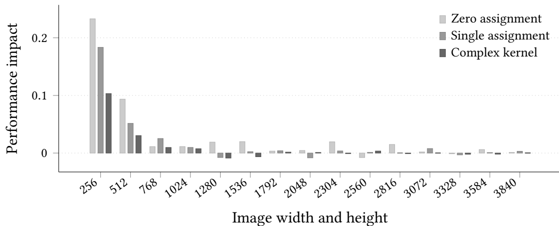
Figure 6.1 Relative performance impact of execution with command queue profiling enabled for two simple and one complex backprojection kernel.
