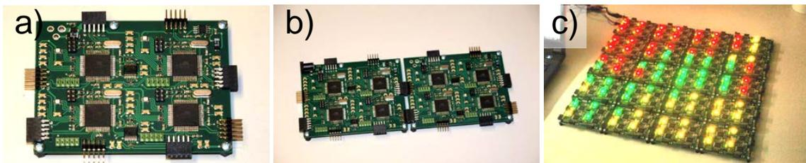
Figure C.2.: Photos of a) a module consisting of four nodes, b) two modules stacked, and c) the Many-Core demonstration platform running AStrA on 80 cores. The platform underlines the feasibility of the proposed approach but was **not** used to obtain any of the presented results!
