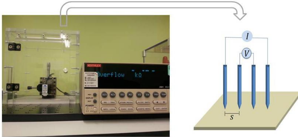
Figure 3.3: Four Probe Point set-up in ICFO used for the sheet resistance measurements (left) and pictorial representation of the four probes on the sample (right).
