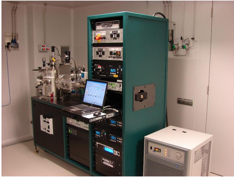
Figure 3.1: The ATC Orion 3 HV sputtering installed in the Nanophotonics Lab, ICFO.
