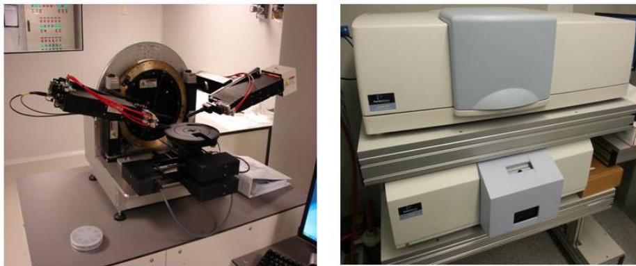
Figure 3.4: Pictures of the ellipsometer set up (left) and the Fourier Transform Infrared Spectrometer (right) used for the experiments at ICFO.
