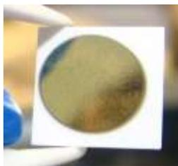
Figure 4.7 Gold sputtered as an electrode on a LATP plate
