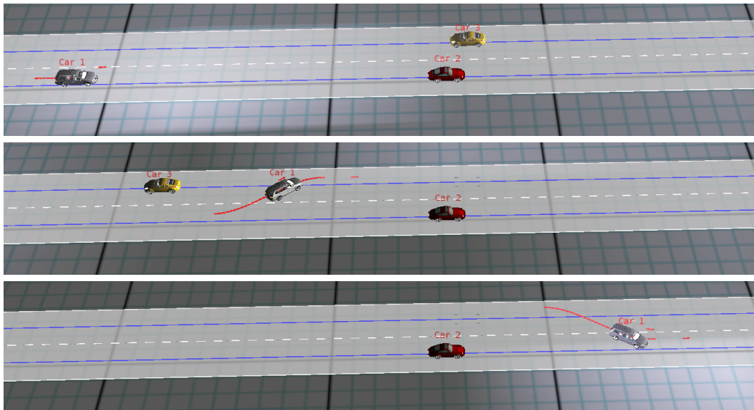
Figure 3.16: Simulation of an overtaking scenario. The policy of the ego vehicle (grey) is derived from solving a corresponding MDP. The planned trajectory is indicated by the red line. (Brechtel et al., 2011).
