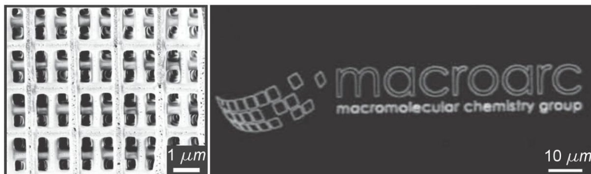
Figure 2.3-7: Scanning electron microscopy (SEM) image of the top of a woodpile structure fabricated via thiol-ene-induced DLW (left). Patterning of the respective three-dimensional structure with a fluorescence maleimide component (right). Images were adapted from Ref. 266 with permission from Wiley.
