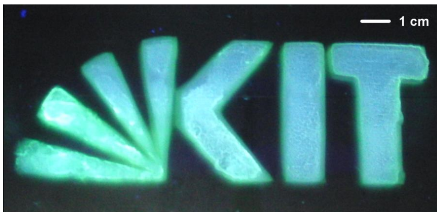
Figure 7.3-5: Image of fluorescent pattern produced by crosslinking a 12/PBD 2 film in the sunlight employing a shadow mask. The fluorescence was visualized using a handheld TLC lamp ( \lambda_{max} = 365 nm).
