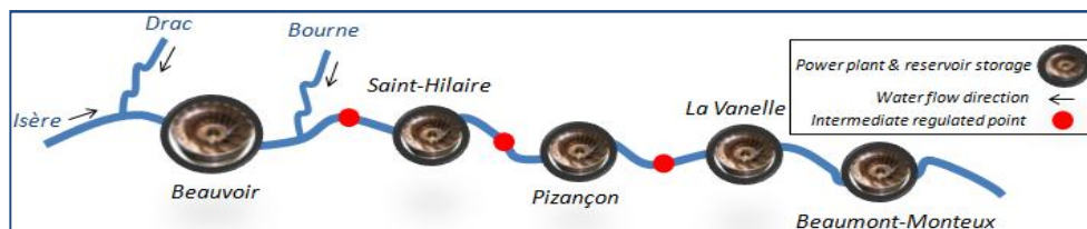
Figure 1: Situation of the HPP located in the lower- Isère valley and participating to Synchronous HydroPeaking function
