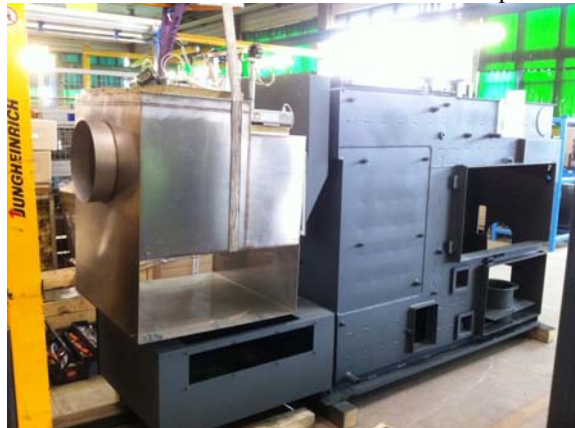
Figure 1: Installation of the electrostatic precipitator at a 200 kW wood-chip boiler
