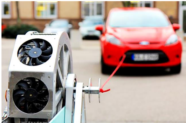
Figure 1: First powerful 'Entropy Wheel' construction developed at the ITCP (KIT) can move a car, 10W mechanical power using hot water at a temperature of 80°C
