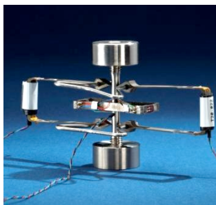
Figure 1: Tensile specimen equipped for Poisson measurement
