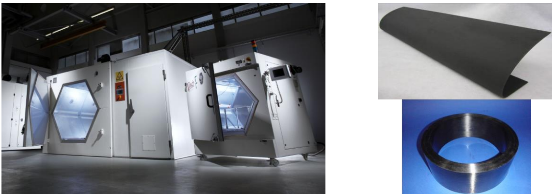
Figure 1: HEPHAISTOS industrial microwave technology and (left) and microwave cured CFRP parts – leading edge via VAP process (top right) and thick wall high precision winding part (bottom right).
