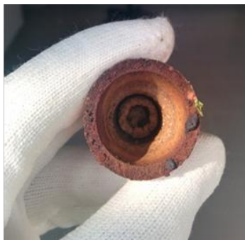
Figure 1: Hydrolysis aspect of the alkali chloride salt and oxides deposition on the container after 6 hours heating at 700 °C with no previous drying procedure.
