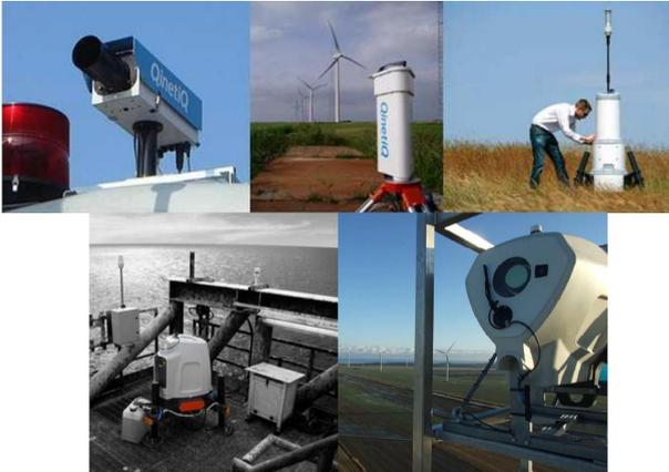
Fig. 3.14: The ZephIR Doppler wind Lidar [70]
