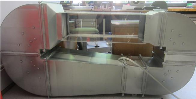
Fig. 6.1: The designed close loop wind tunnel
