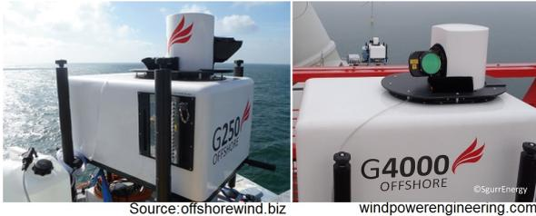
Fig. 3.22: Galion Lidar G250 and G4000 (Source: Sgurr Energy)
