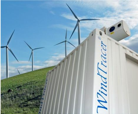
Fig. 3.26: WindTracer Lidar system (Source: Lockheed Martin)
