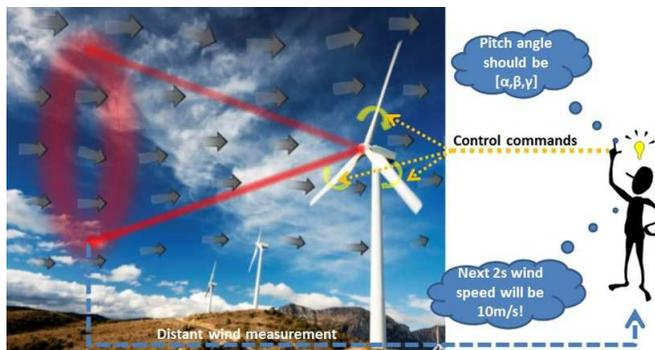
Fig. 4.: Sketch of the general idea of Lidar assisted wind turbine pitch control system (Background picture source: Microsoft office template)
