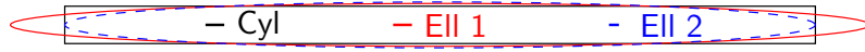
Figure 4.11: Approximation of a cylindrical fiber with equal volume and aspect ratio or volume and length
