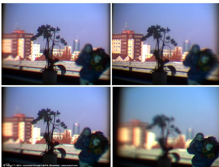
Fig. 8. Series of 4 images taken from a depth-extended scene. The optical setup targets objects that are separated at three distances from the optical system: far, intermediate, and near. For each of the images, both the focus and the pivot axis are readjusted.
