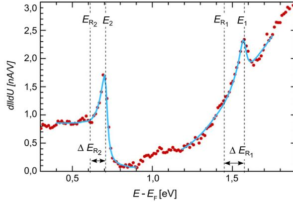
**Figure 3.** Tunneling spectrum (red dots) of the  $(\sqrt{3} \times \sqrt{3})$  Pb/Ag(111) $R30^\circ$  surface alloy showing two peaks at  $E_1 = 1580$  meV and  $E_2 = 710$  meV (set point:  $I_{\text{set}} = 1$  nA,  $U_{\text{set}} = -1$  V). The blue lines represent fits to the peaks (see text for details).
