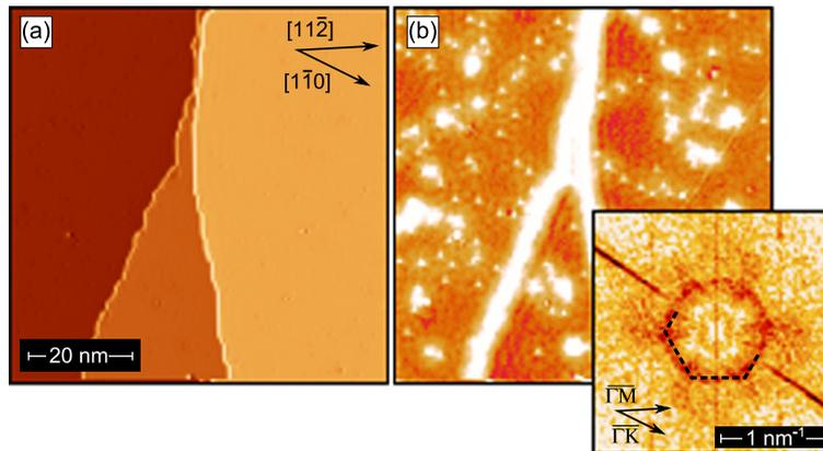
**Figure 5.** (a) Constant-current image of the  $(\sqrt{3} \times \sqrt{3})$  Pb/Ag(111) $R30^\circ$  surface alloy. (b)  $dI/dU$  map measured at  $U = 1037$  mV. The inset shows the corresponding two-dimensional Fourier-transformation of (b).
