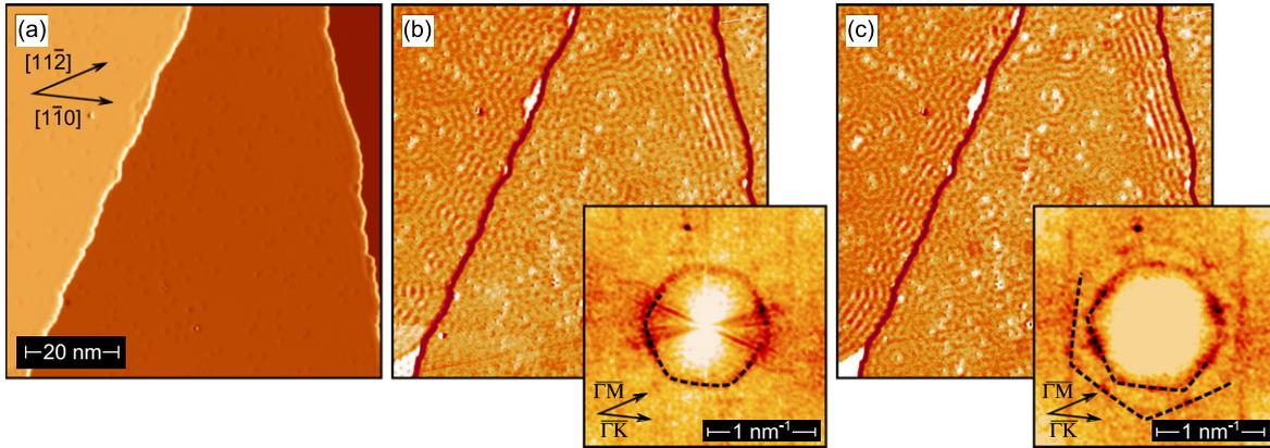
**Figure 4.** (a) Constant-current image of the  $(\sqrt{3} \times \sqrt{3})$  Pb/Ag(111) $R30^\circ$  surface alloy. (b)  $dI/dU$  map measured at  $U = -163$  mV and (c) at  $U = -263$  mV. The insets show the corresponding Fourier-transformed (FT)  $dI/dU$  maps. The hexagonal shape of the FT depicts the anisotropic dispersion along the  $\overline{\Gamma K}$  and  $\overline{\Gamma M}$  directions.
