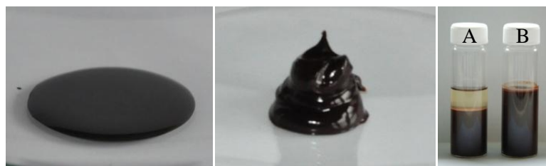
Figure 21: Suspension of \phi=0.35 cocoa solids in oil suspension without added water ( S = 1.0 , left) and with added water ( S = 0.90 , middle). Right image: sedimentation behavior after a storage time of 5 days, (A) no water added, (B) S = 0.90 .
