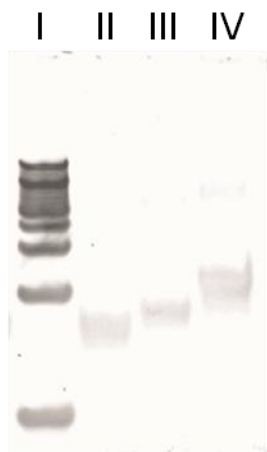
Figure 22. 21% TBE gel electrophoresis of I: 10 base pair marker, II: amino-DNA 81 , III: Mal-DNA 83 and BTPE+Mal-DNA 84 after 2 h 15 min at a voltage of 100 V using SYBR Gold staining.
