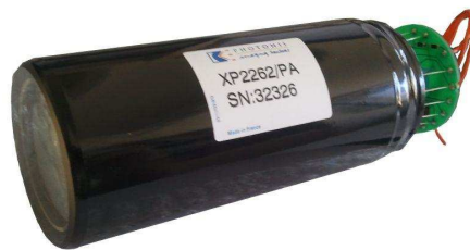
Figure 4.5: The XP-2262 PMT. The voltage divider circuit board is visible on the right side, connected to the PMT.
