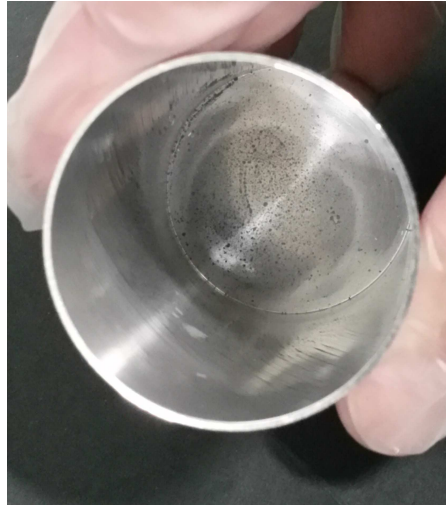
Figure 5.24: The oxidized inner surface of the aluminum cup.
