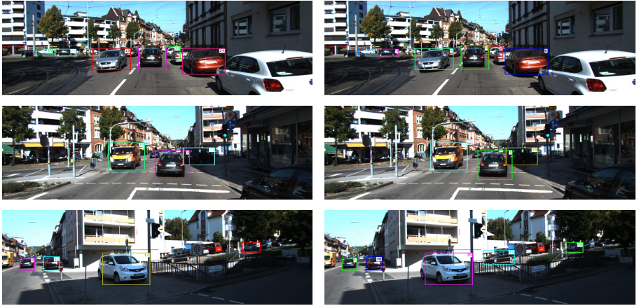
Figure 6.23: RESULTS FOR THE OPTIMAL (LEFT) AND APPROXIMATIVE SOLUTION (RIGHT). Preceding objects in crowded scenes are tracked continuously. The preceding (black) car is followed for 9.5s
