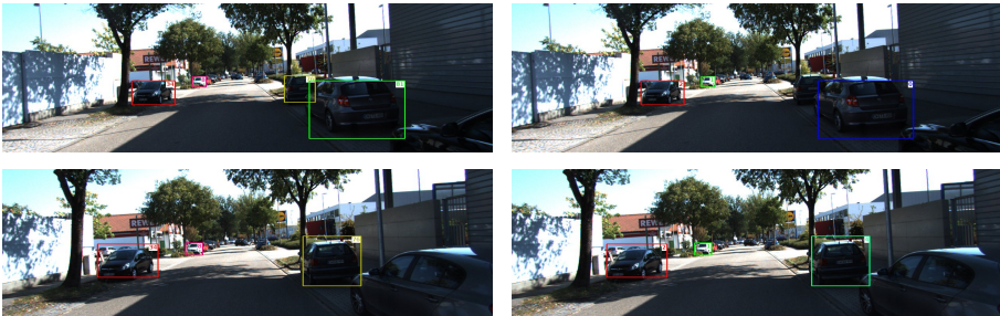
Figure 6.26: RESULTS FOR THE OPTIMAL (LEFT) AND APPROXIMATIVE SOLUTION (RIGHT). Missing future evidence for the approximative solution may lead to tracks starting later compared to the optimal solution (second car on the right). This happens primarily for detections with a low score for the early part of the trajectory.
