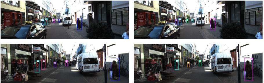
Figure 6.27: RESULTS FOR THE OPTIMAL (LEFT) AND APPROXIMATIVE SOLUTION (RIGHT). For crowded inner-city scenes, objects of different classes (cars, pedestrians, cyclists) are tracked robustly over the main part of their presence in the image.
