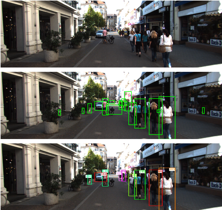
Figure 1.2: MULTI-TARGET TRACKING STAGES: For the given input data (top), an object detector returns different types of traffic participants (middle), and object tracks are established for the input sequence discarding outliers (bottom).
