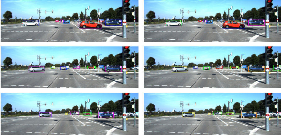
Figure 6.25: RESULTS FOR THE OPTIMAL (LEFT) AND APPROXIMATIVE SOLUTION (RIGHT). Challenging intersection scenarios lead to qualitatively good results. The limited optimization window for the approximative solution may also avoid fragmentations of the trajectory outside of this window.
