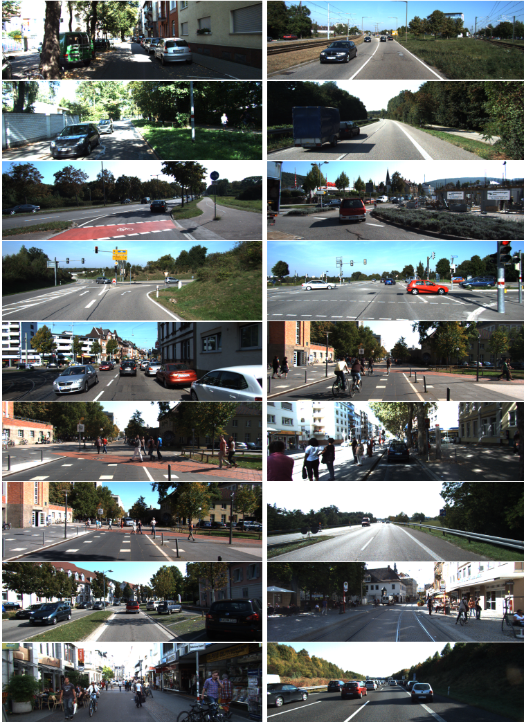
Figure 6.11: ILLUSTRATION OF THE DATASET. This figure exemplarily shows 18 images selected from the 50 sequences compiling the KITTI tracking benchmark. For all sequences grayscale and color stereo images, laser point clouds, GPS/IMU information, and calibration matrices are available. Note the wide variety and complexity of scene types, quantitatively stated in Fig. 6.9d.
