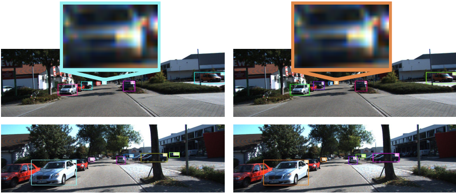
Figure 6.21: RESULTS FOR THE OPTIMAL (LEFT) AND APPROXIMATIVE SOLUTION (RIGHT). Far away objects are tracked continuously. The oncoming car is followed for 3.7s and not confused with several parking cars.
