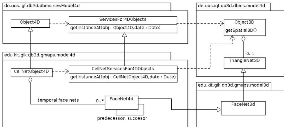
Fig. 93: The extraction of a 3D face net from a temporal cell net object as class diagram
