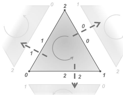
Fig. 60: Indexing of net topology in DB4GeO triangle net component
