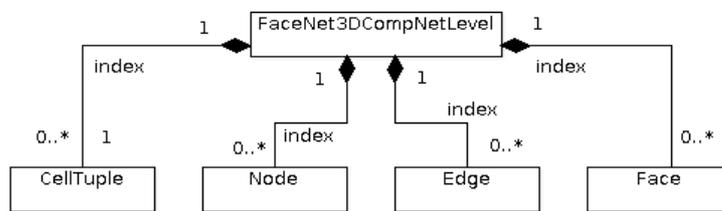
Fig. 51: FaceNet3DCompNetLevel as composition of indices of CellTuple objects and cells
