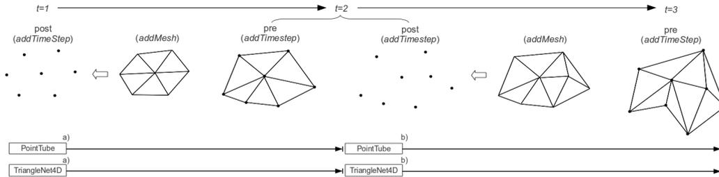
Fig. 90: Example of creation of temporal objects with DB4GeO Temporal Joint Model
