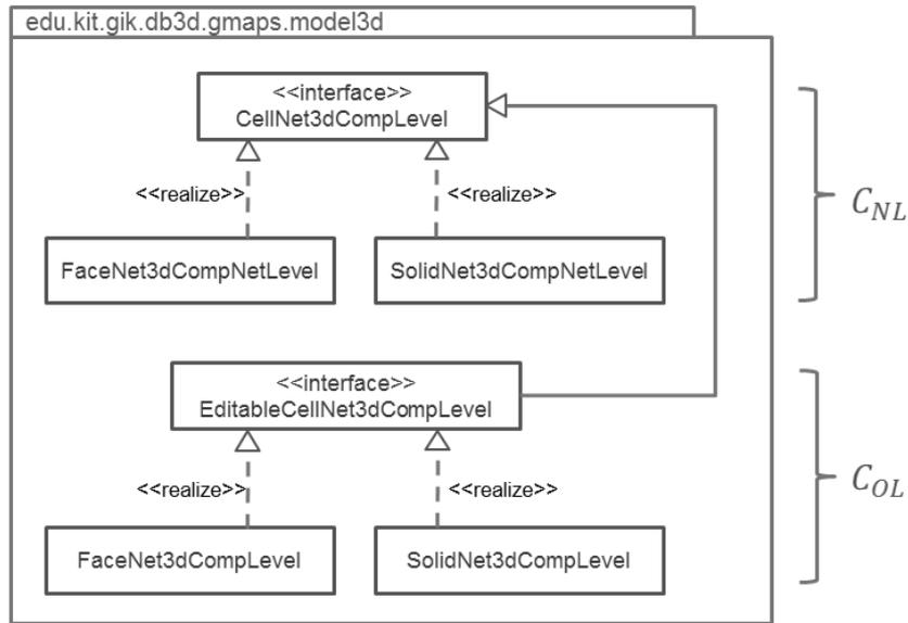
Fig. 56: Two distinctive cell net component interfaces
