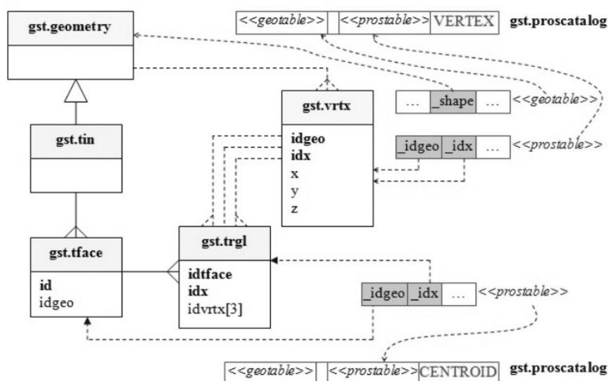
Fig. 5: TIN part of the relational data model of GST
