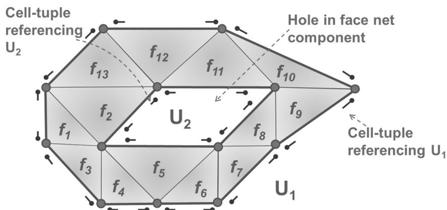
Fig. 52: Face net component in outer void ( $U_1$ ) with additional inner hole ( $U_2$ )
