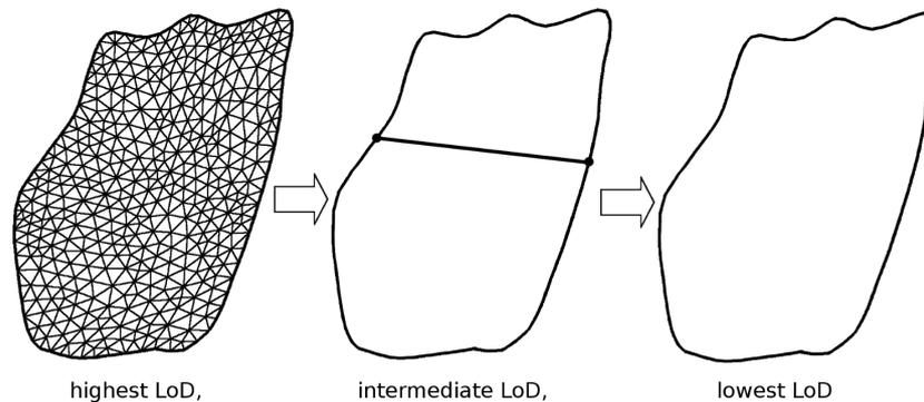
Fig. 26: A subsurface fault, depicted in three levels of detail
