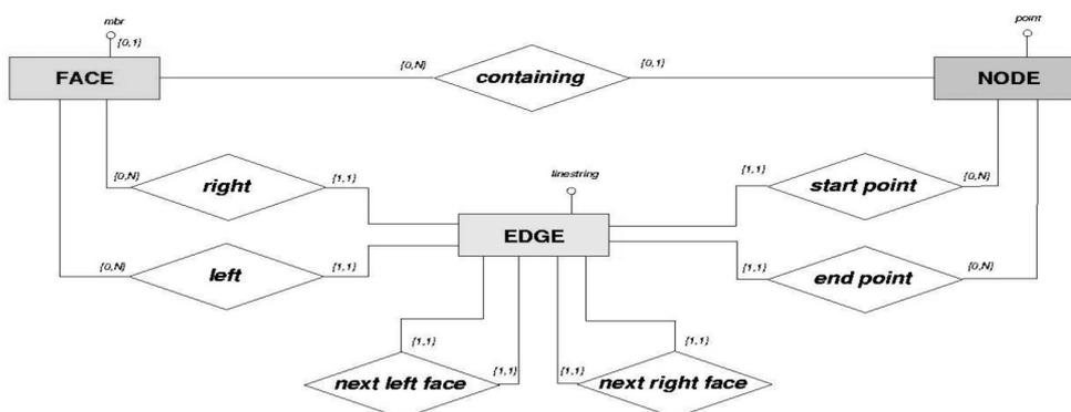
Fig. 4: Conceptual PostGIS topology model
