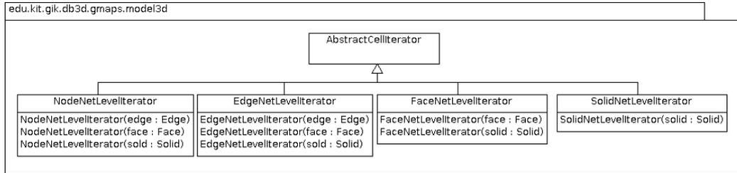
Fig. 71: Closure cell iterator classes
