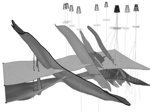
Fig. 2: Typical subsurface model with two strata boundary layers, seven fault layers and visualized well data
