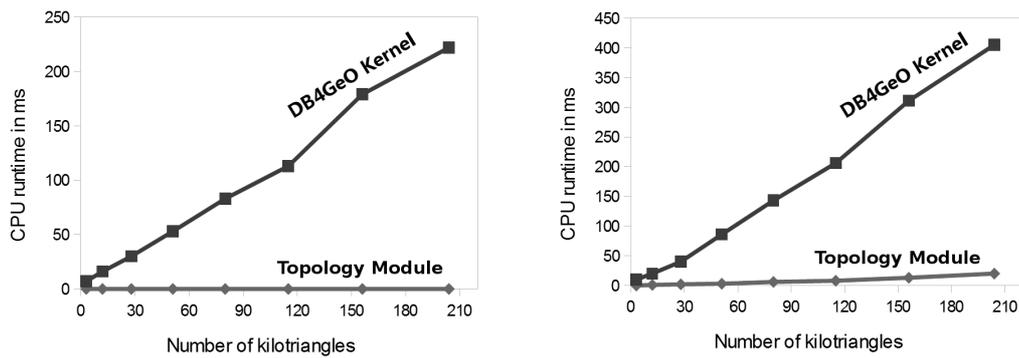
Fig. 103: Runtimes of *get-1D-for-0D* operations (left); runtimes of *countBorderEdges* operations (right)
