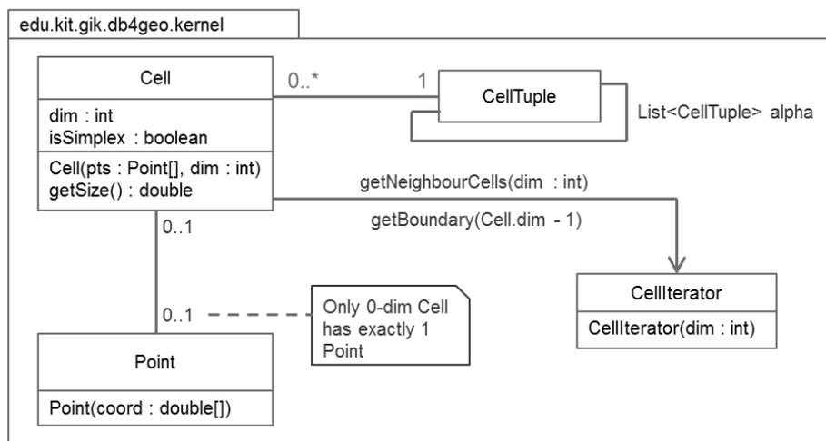
Fig. 107: Classes of dimension-independent cell model approach
