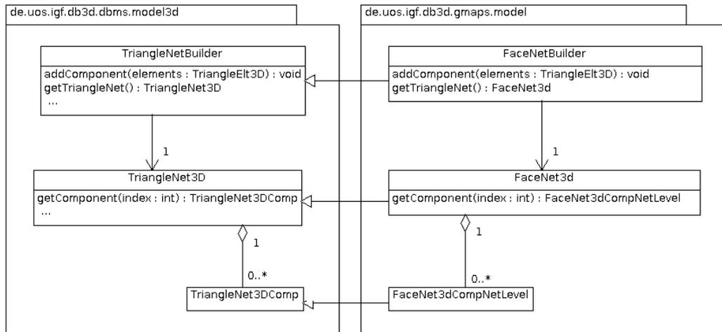
Fig. 49: Face net builder architecture as an extension of the triangle net builder architecture of DB4GeO
