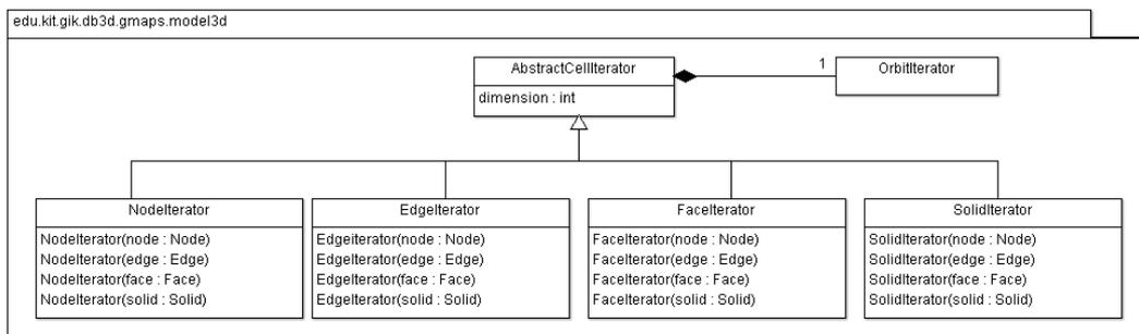
Fig. 68: Boundary cell iterator classes
