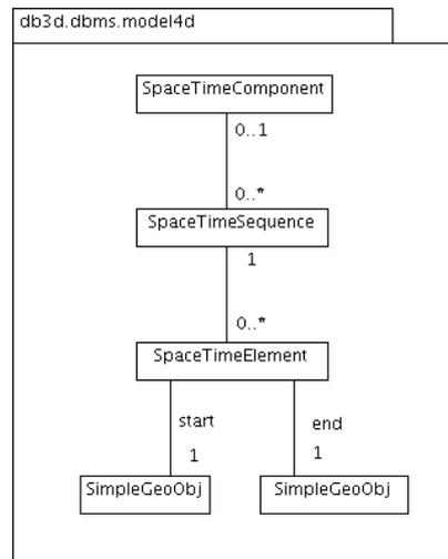
Fig. 31: Simplified UML diagram of the space-time model of DB4GeO/DB3D
