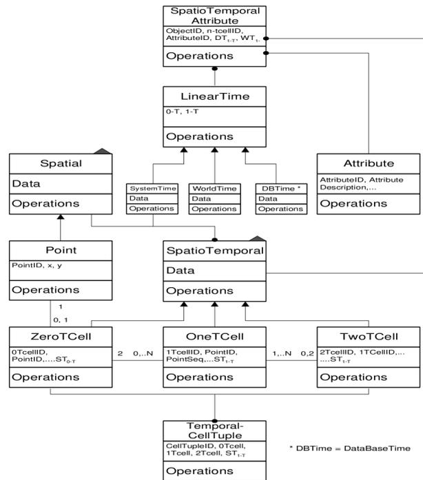
Fig. 35: Cell tuple based spatio-temporal data model
