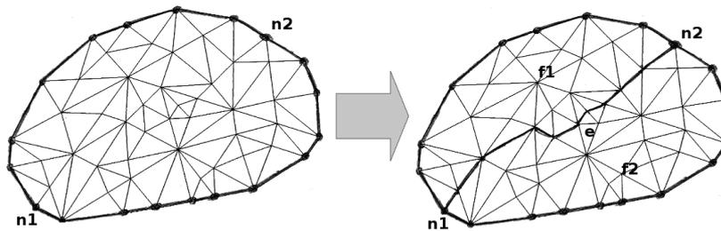
Fig. 79: Example of insertEdge operation, represented on object and on net level
