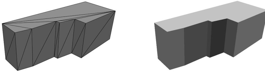
*Fig. 105: Net level and object level representation of building model*
