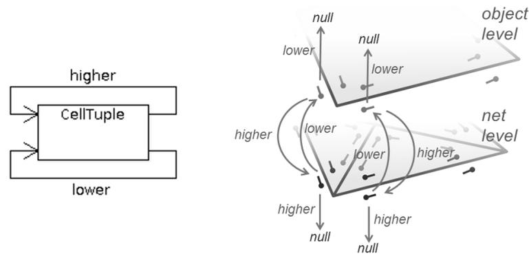
Fig. 57: Higher and lower field attributes of `CellTuple` class (left: class diagram; right: example set-up)
