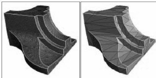
Fig. 23: Application of the progressive mesh algorithm (left: a geometric object in full detail; right: the same object with reduced detail)
