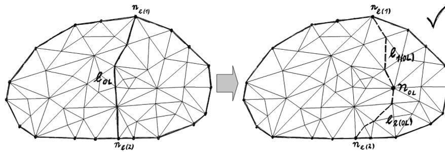
Fig. 76: Example of `insertNode`, represented on object and on net level (left: before operation, right: after operation)
