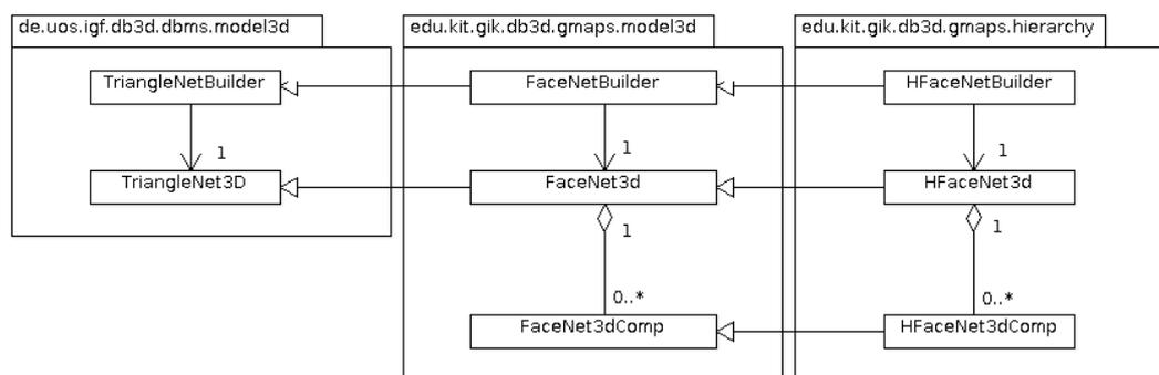
Fig. 84: Architecture of hierarchical net builder as an extension of the cell net builder architecture
