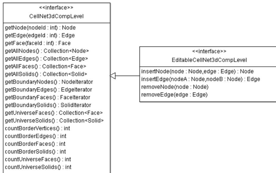
Fig. 58: Cell net comp level methods
