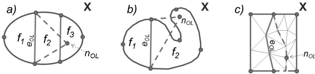
Fig. 77: Examples of illegal states for `insertNode` method
