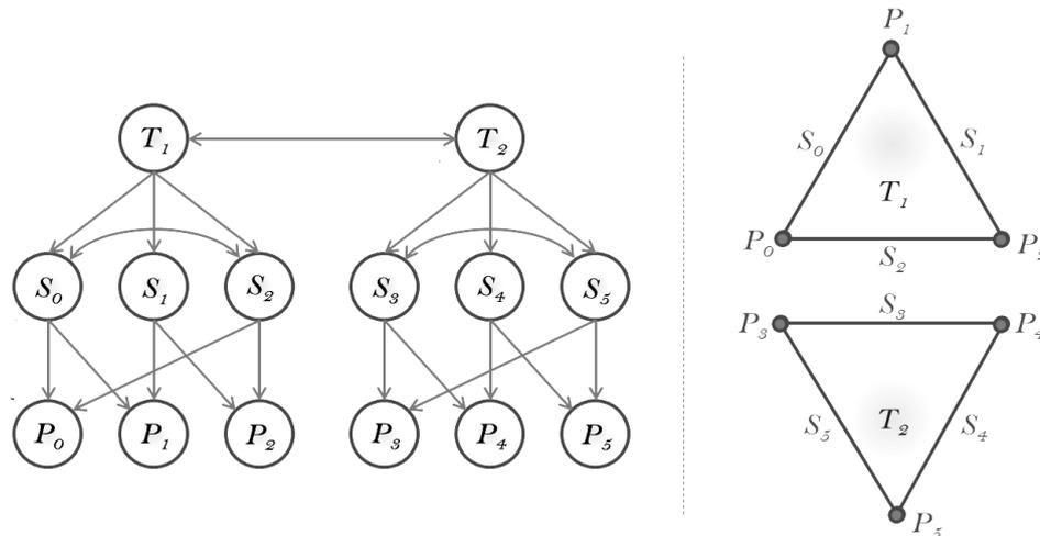
Fig. 18: Incidence graph of Simplicial Complex model of the DB4GeO kernel (T: triangle, S: line segment, P: point)
