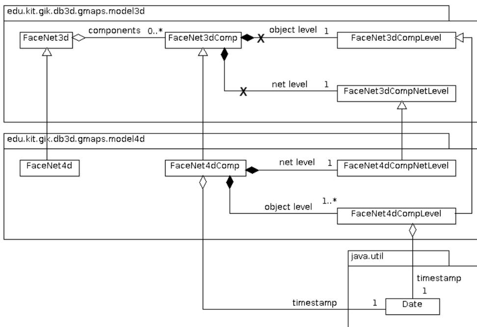
Fig. 96: The temporal net components (with their NL and OL) of temporal face nets in a class diagram
