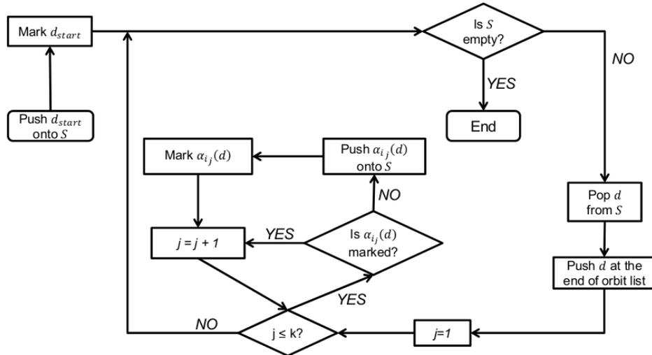
Fig. 22: Flow chart diagram of dimension independent orbit traversal algorithm
