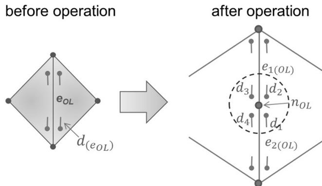
Fig. 78: Adding new cell-tuples when performing `insertNode` method
