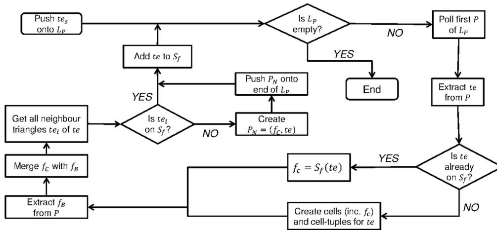
Fig. 59: Flow chart diagram of `cellNetBuildUp` method
