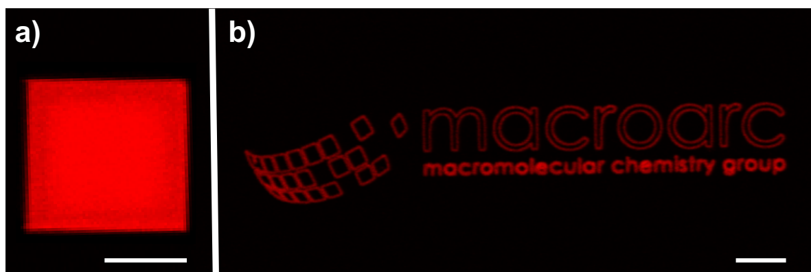
Figure 3.11: LSM images of structures fabricated by radical thiol-ene mediated DLW after subsequent immobilization of fluorescein maleimide via a thiol-Michael addition procedure. A woodpile structure is displayed in a) while the macroarc group logo is depicted in b). The scale bar for both images is 10 \mu\text{m} .
