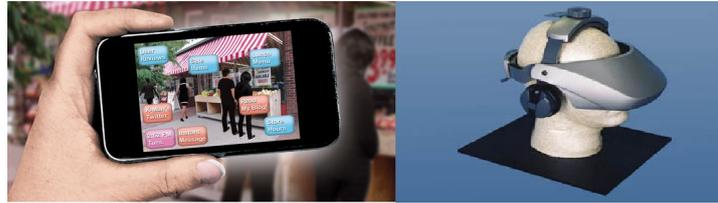
**Fig. 1.** a head mounted display (a) on the left and a handheld device (b) on the right which is used to display the AR system.
