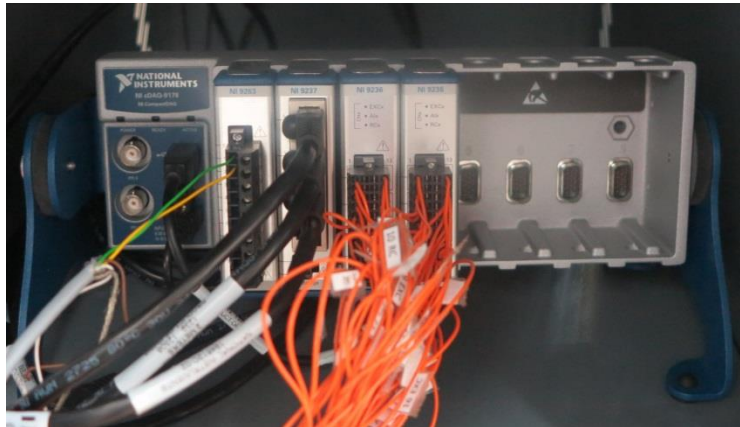
Figure 6.6: Modular data acquisition system CompactDAQ
