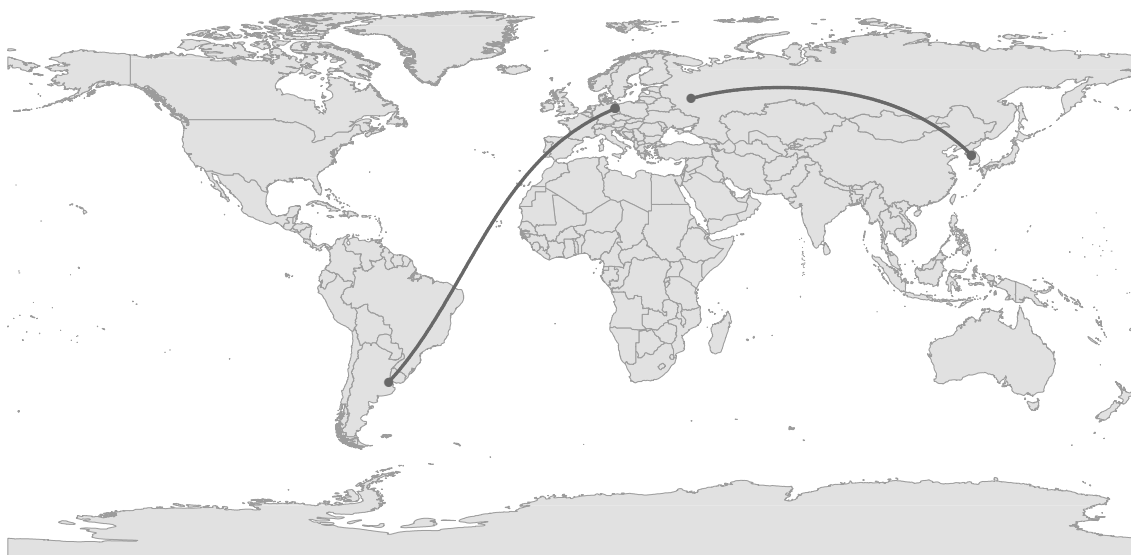
Figure B.2: Great Circle Distances between Berlin and Buenos Aires and between Moscow and Seoul on a Plate Carée Projection of the Earth.
