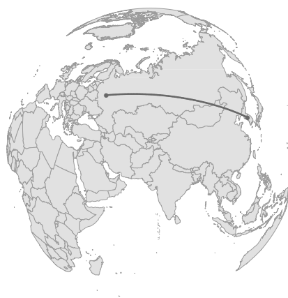
(b) Great Circle Distance between Moscow and Seoul on the Surface of a Spherical Earth.
