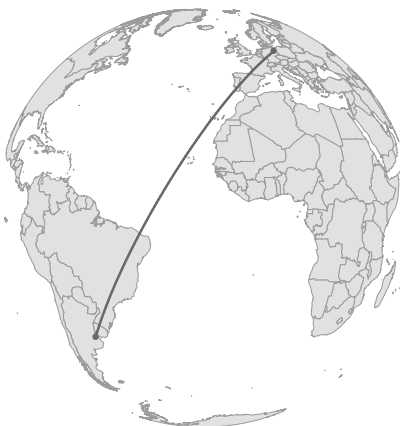
(a) Great Circle Distance between Berlin and Buenos Aires on the Surface of a Spherical Earth.
