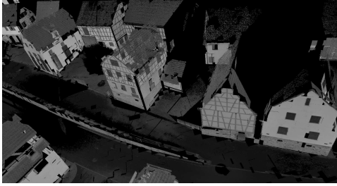
Figure 2. Point clouds of a Z+F sensor colored by intensity.
