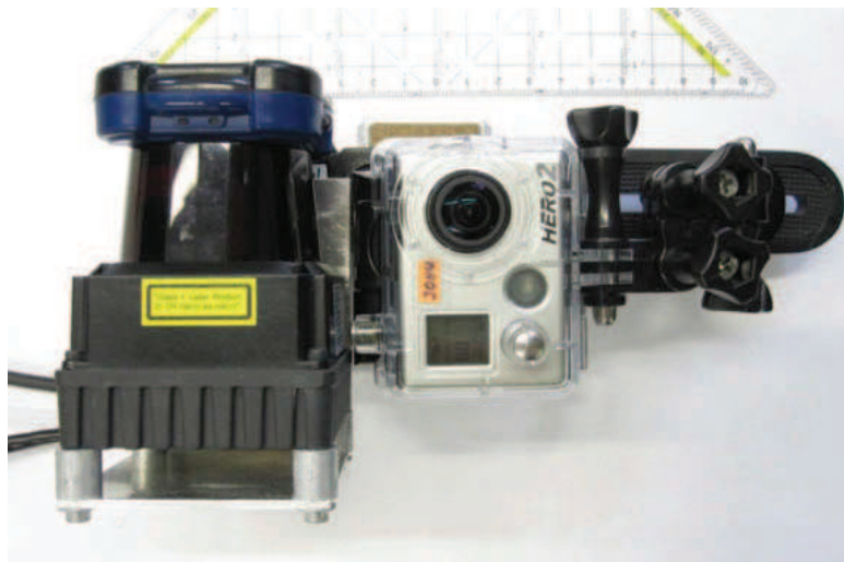
Figure 1. Sensor platform with two sensors: laser scanner (left: Hokuyo UTM-30LX-EW) and digital camera (right: GoPro 1080p HD HERO2).
