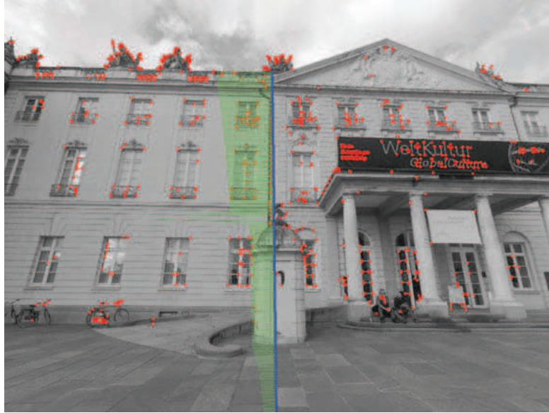
Figure 4. First image of the sequence captured in front of the Karlsruhe Palace (red: extracted salient image points; blue: laser points projected onto the image; green: scaled representation of range measurements).
