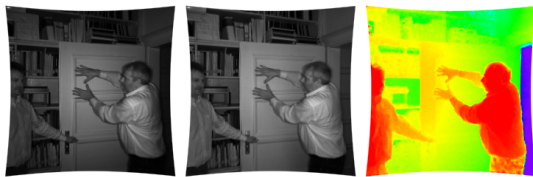
Figure 4: Visualization of the undistorted images for normalized active intensity, normalized passive intensity and range information (from left to right).
