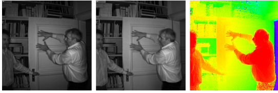
Figure 2: Visualization of the data captured with a PMD[vision] CamCube 2.0: Normalized active intensity image, normalized passive intensity image and range image (from left to right). The range is encoded in terms of a color scale reaching from red (near) via yellow, green, cyan and blue to violet (far).
