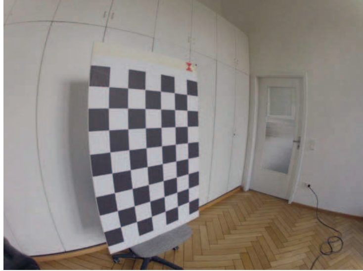
Figure 2. Example of a distorted image with a calibration plane (checkerboard).
