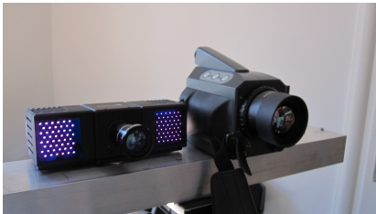
Figure 10: Sensor platform equipped with a range camera (left) and a thermal camera (right).
