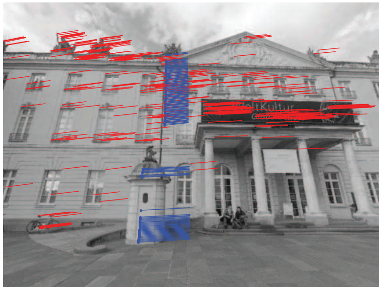
Figure 5. The result for the tracking from the second to the third image using the features extracted at the first pose (red: tracked salient image points; blue: tracked laser points).
