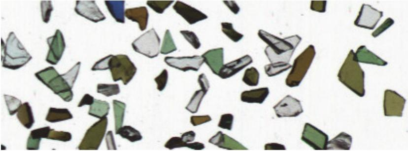
**Figure 5.1:** Photo of real glass shards obtained by a line scan camera of an AOI image acquisition system (courtesy of Fraunhofer IOSB).
