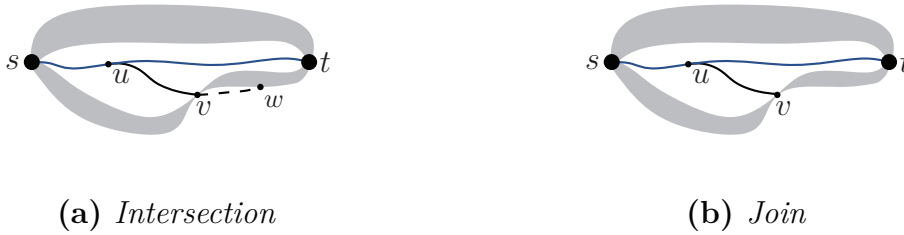
Figure 8.1: Consideration of a path to use in an alternative graph. The left side shows a segment that leaves the shortest path at u , crosses the alternative graph at v and joins it at w . On the right side, the path joins the corridor directly at v . By considering all segments between corridor vertices individually ( (u, v) and (v, w) are treated separately of each other), we might end up keeping only the first part of the deviation for our alternative graph. The latter segment is discarded if it does not constitute a viable deviation on its own. As a result, both paths, though different, could end up contributing the same to the alternative graph.
