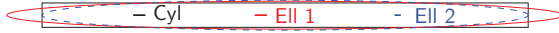
Figure 4.11: Approximation of a cylindrical fiber with equal volume and aspect ratio or volume and length
