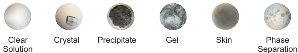
Figure 4: Proteins can undergo phase transitions into different phase states: clear solution (soluble), crystal, precipitate, gel, skin, and liquid-liquid phase separation.
