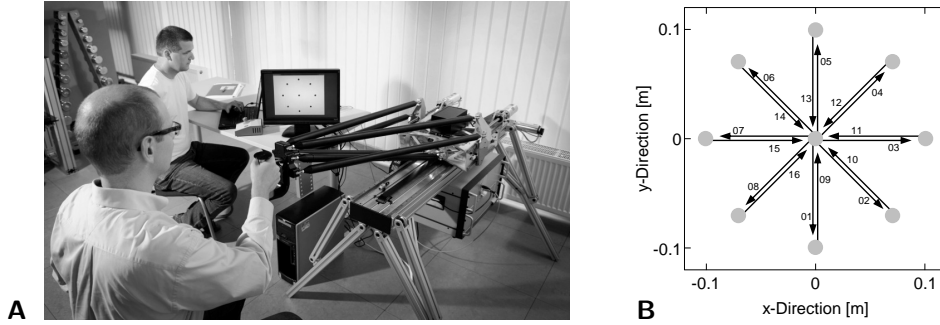
Figure 2.1: Classical two-dimensional center-out movement task. A , Subject performing center-out movements handling the robotic manipulandum BioMotionBot. The cursor representing the position of the handle and the target points are visualized on a screen. B , The center-out movement task typically comprises movements from a center point to circumjacent target points and back.
