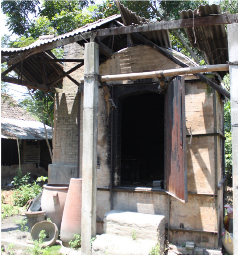
Figure A 8: Advanced kiln in Kasongan which could be restored and used for filter production
