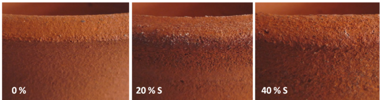
Figure A 11: Surfaces of ceramic filter pots made of 0, 20 and 40 % saw dust.
