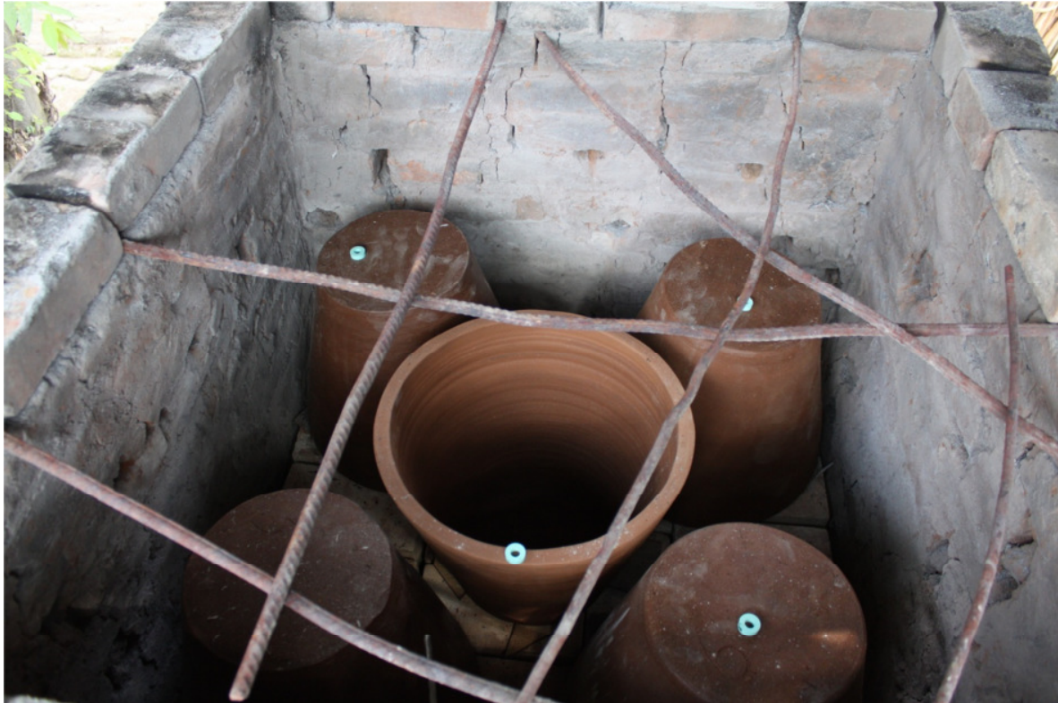
Figure A 9: Pots in the traditional kiln before firing. Kiln is still open. Greenish process temperature control rings are distributed on each side on top of the pots and at the bottom of the kiln.
