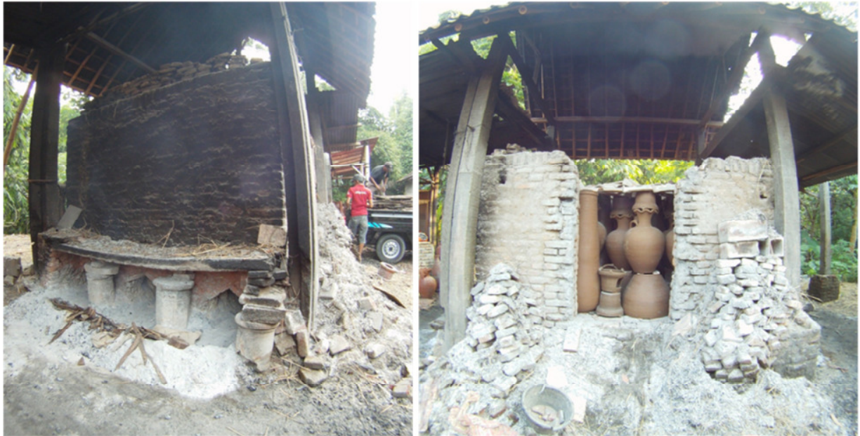
Figure A 7: Covering of the kiln. Left: front is sealed with bricks and plaster. Middle: covering of the kiln before firing. Right: after firing.
