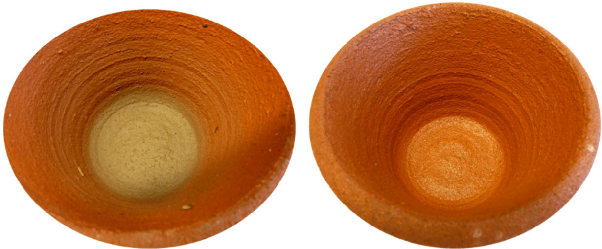
Figure 33: 40 % rice husk filter after filtering brook water (left) and after subsequent cleaning (right)
