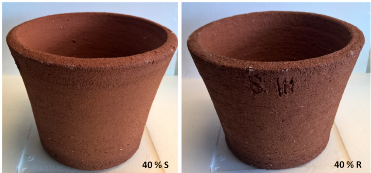
Figure A 11: Surfaces of ceramic filter pots made of 0, 20 and 40 % saw dust.
