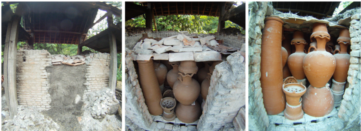
Figure A 7: Covering of the kiln. Left: front is sealed with bricks and plaster. Middle: covering of the kiln before firing. Right: after firing.
