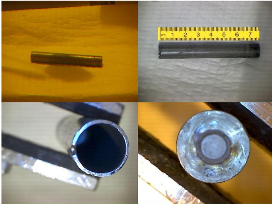
**Figure 4.3:** Pictures and dimension of the irradiated plenum Zircaloy-4. The upper two pictures show the whole irradiated Zircaloy-4 plenum specimen. The lower left picture shows the bottom half of the specimen, where the plenum was cut from the fuel rod segment whereas the lower right picture shows the massive Zircaloy-4 end cap of the plenum specimen.
