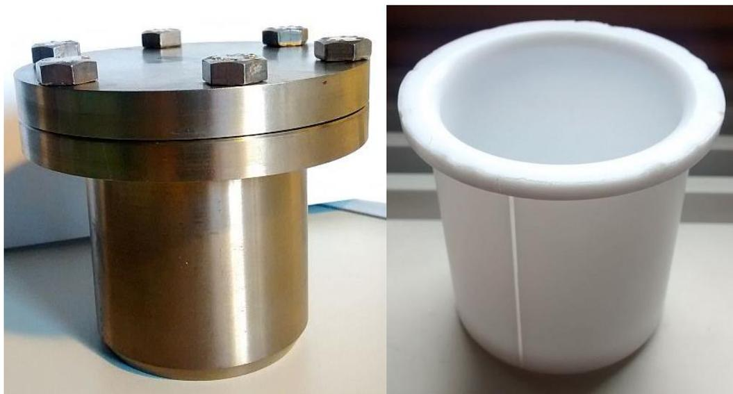
**Figure 4.1:** Images of the autoclave and PTFE liner used for the hydrothermal preparation of  $\text{Nd}(\text{OH})_2\text{Cl}(\text{s})$  at  $80^\circ\text{C}$ . The picture on the left shows the autoclave itself whereas the picture on the right shows the PTFE liner used in the autoclave.
