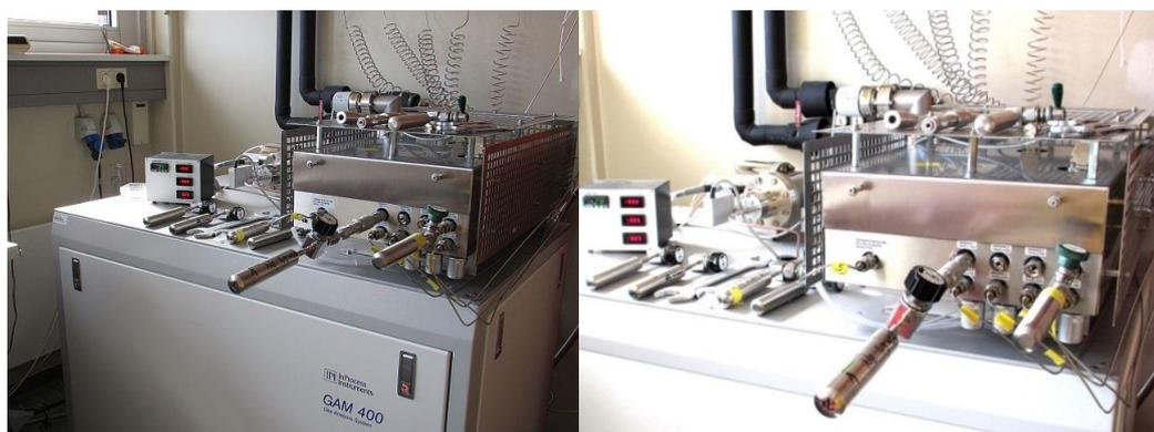
**Figure 4.6:** Pictures of GAM400 quadrupole gas-MS and the batch inlet system for connecting the gas collecting cylinder to the instrument.
