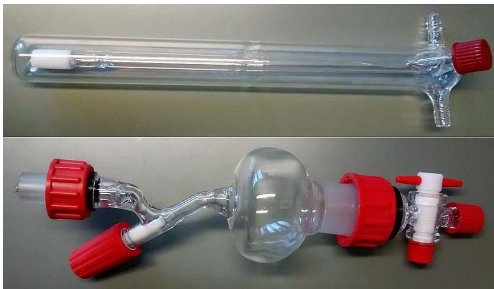
**Figure 4.10:** Customized washing bottle (250 mm × 20 mm) equipped with a fritted glass tip of porosity 1 (upper picture) and customized dropping funnel (120 mL, lower picture).
