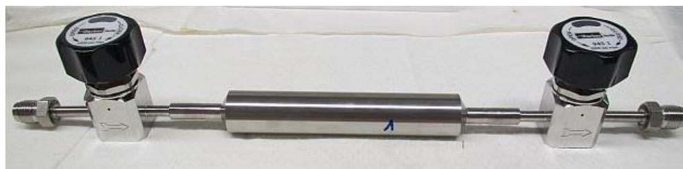
**Figure 4.13:** Double-ended gas collecting cylinder for gaseous samples derived from digestion experiments with Zircaloy-4 performed in an autoclave.
