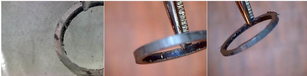
**Figure 5.14:** Black/blueish precipitates seen on the inner surface of the irradiated Zircaloy-4 cladding.
