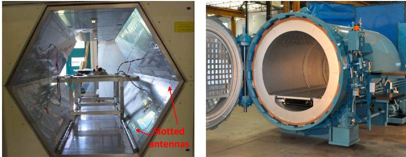
(a) Photo of HEPHAISTOS. (b) Autoclave in CFRP curing [aut].
