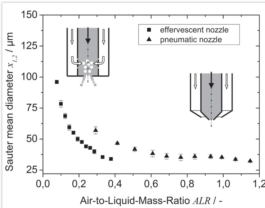
Figure 4: Impact of ALR on the Sauter mean diameter of the spray droplets atomized by an external mixing pneumatic nozzle and an effervescent atomizer at constant liquid flow (liquid viscosity: 25.5 mPas) [6]
