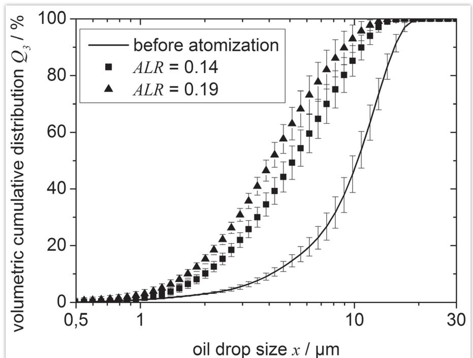
Figure 5: Oil drop size distribution of an oil in water emulsion before (continuous line) and after atomization (discrete data points) by an effervescent atomizer at two different ALR [7].
