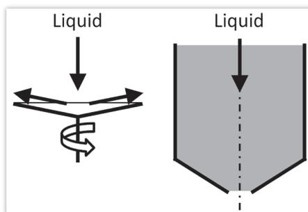
**Figure 1: Schematic drawing of a rotary atomizer (left) and a pressure nozzle (right).**
