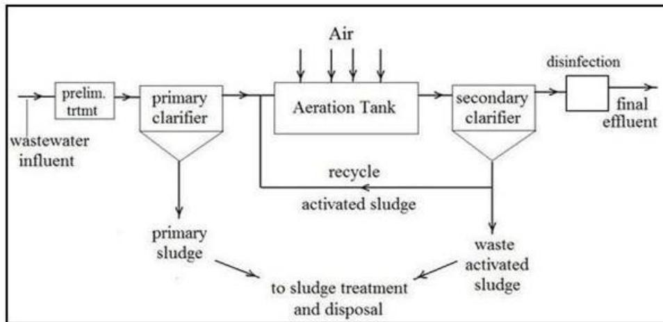
**Figure 1:** Activated sludge waste water treatment flow diagram.
