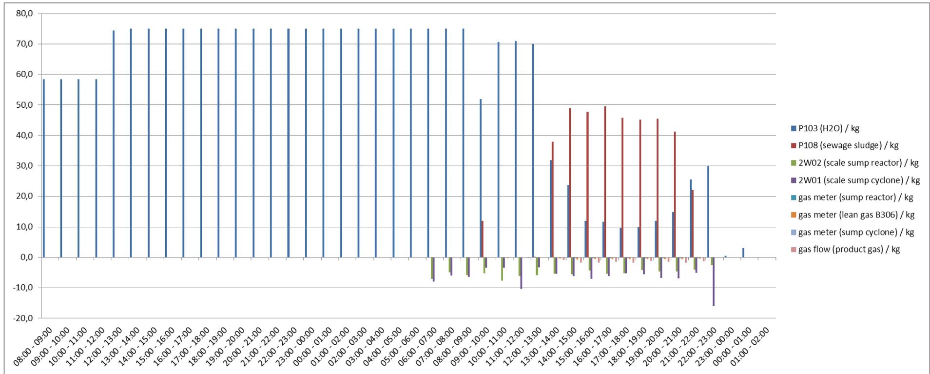
**Figure 15: IN streams (positive values) and OUT streams (negative values) of the VERENA test KS-1 (without the effluent water) for the whole experimental time (including the heat up phase).**
