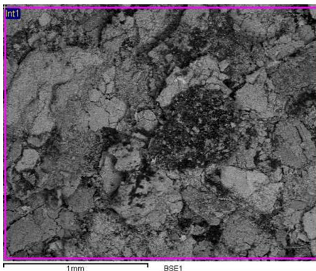
**Figure 17: REM-picture of some solid residue in the VERENA plant (corrosion).**
