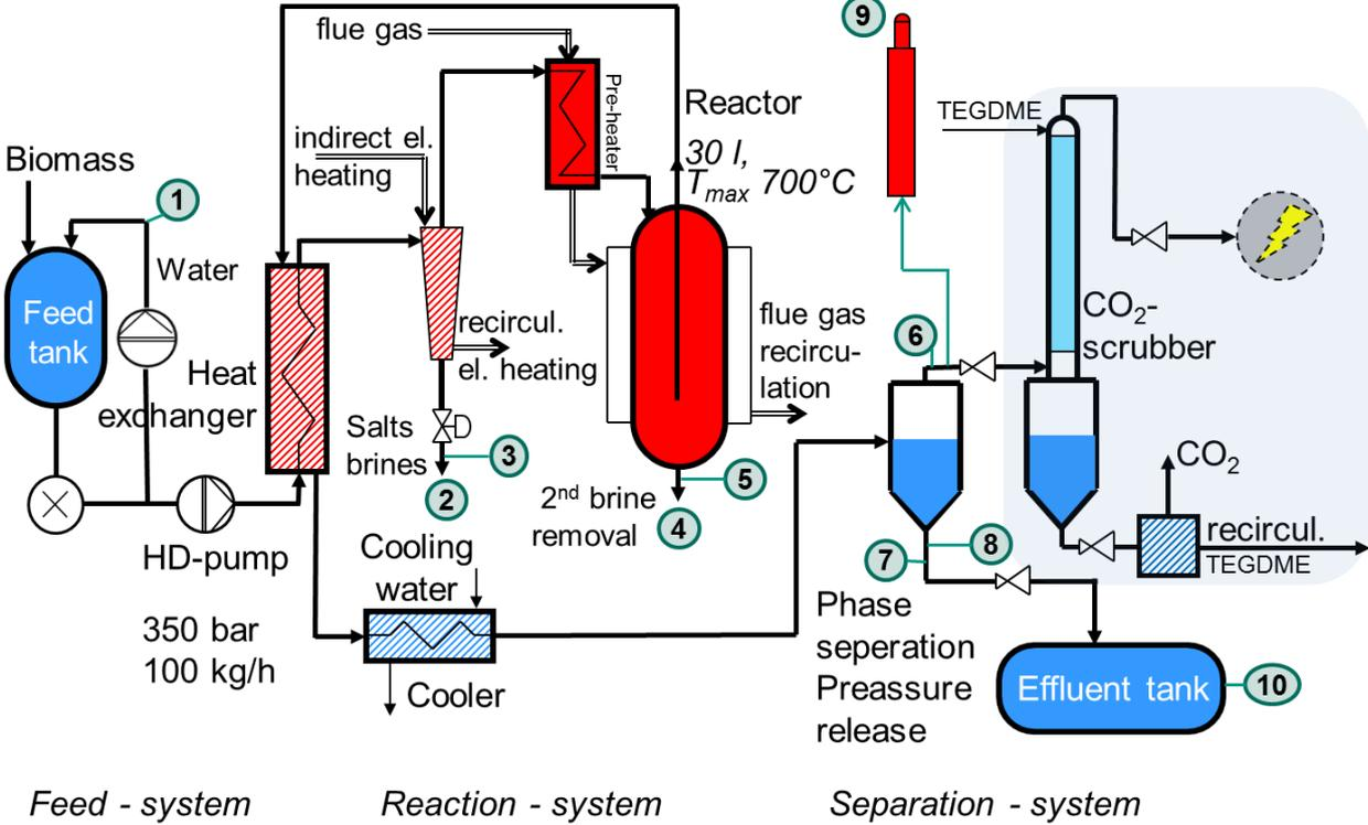
Figure 2: Pilot plant VERENA – flow sheet.
