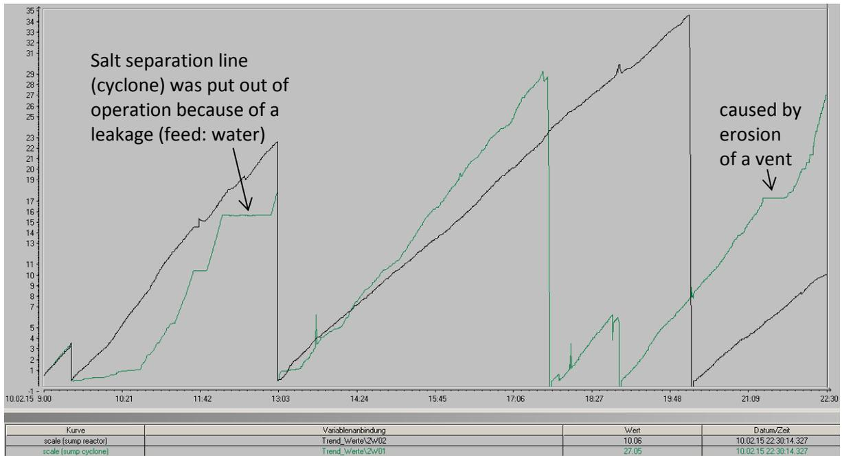
Figure 12: Sum of the salt concentrate separated from the sump of the cyclone (green) and from the sump of the reactor (black) in kg.
