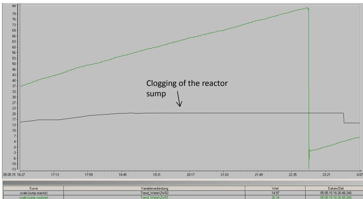
Figure 23: Sum of the salt concentrate separated from the sump of the cyclone (green) and from the sump of the reactor (black) in kg during steady state phase.
