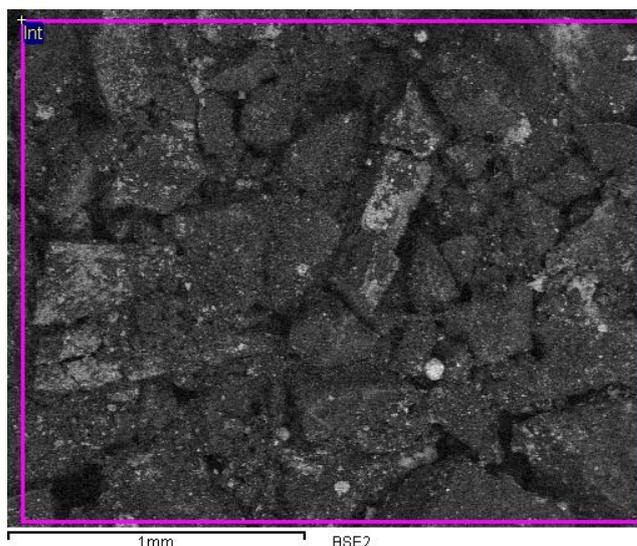
**Figure 16: REM-picture of the residue of the plugging in the VERENA plant.**
