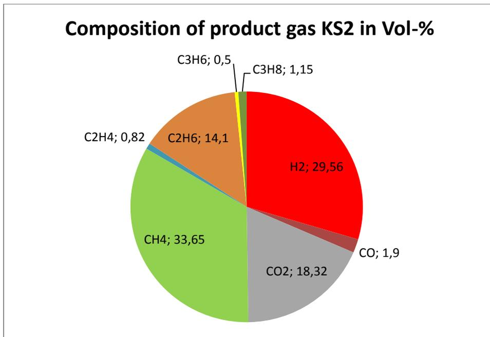
**Figure 25: Composition of the product gas of experiment KS2.**
