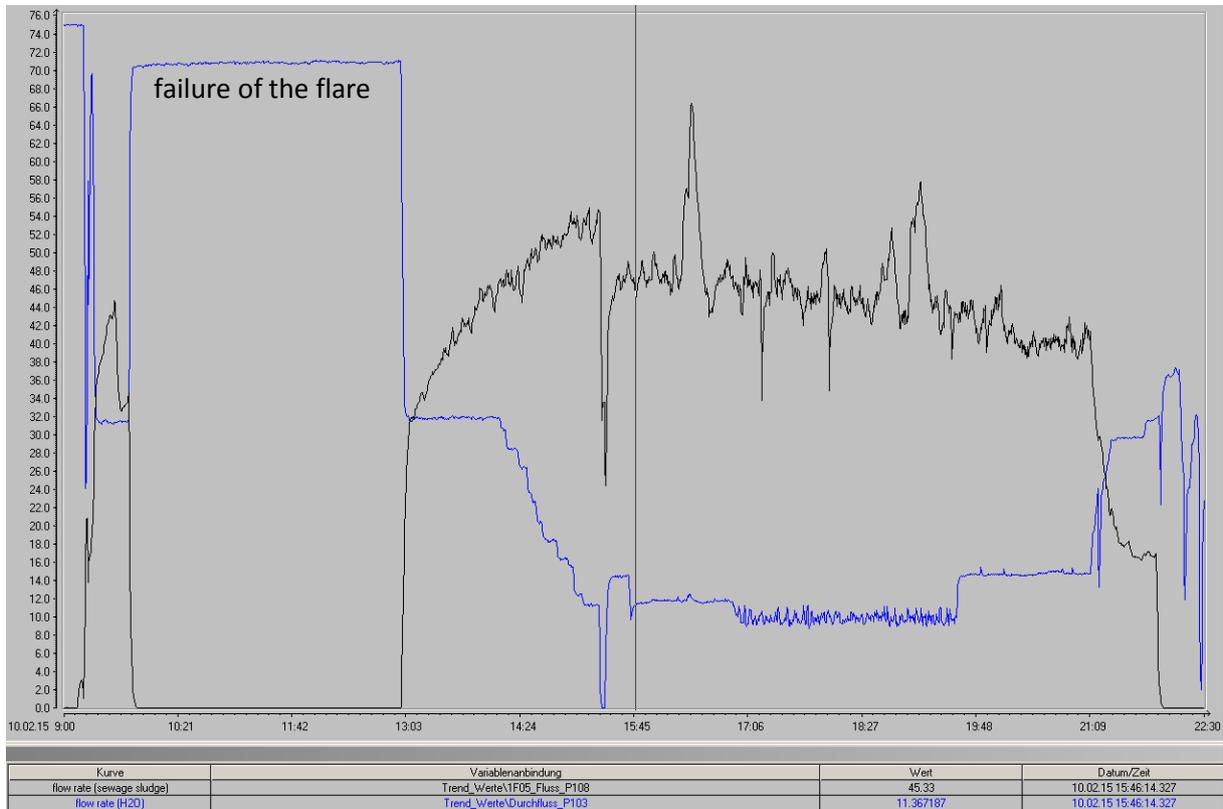
Figure 10: Feed stream of the VERENA test in kg/h.
