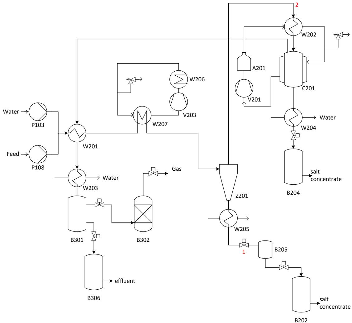
**Figure 8: Process flow sheet of the VERENA plant (the buffer tank B205 was first implemented for the second pilot-scale experiment)**
