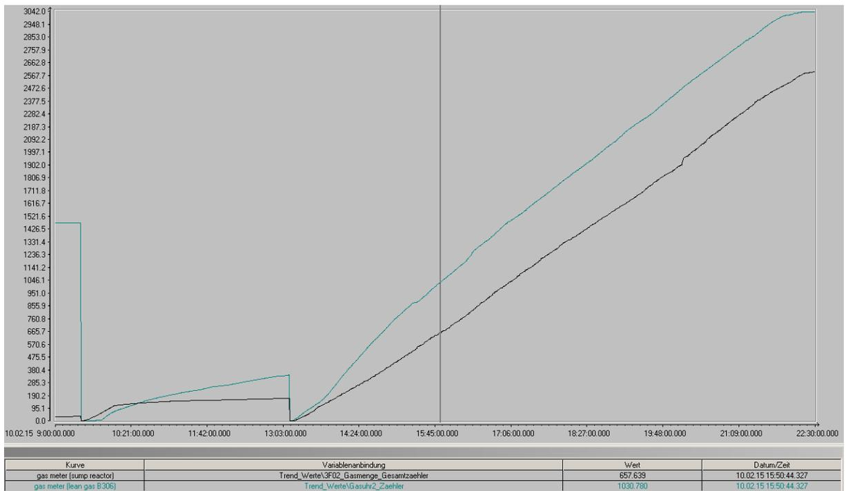
Figure 13: Sum of the lean gas from the waste water (turquoise) and the salt concentrate separated from the sump of the reactor (black) in liter.
