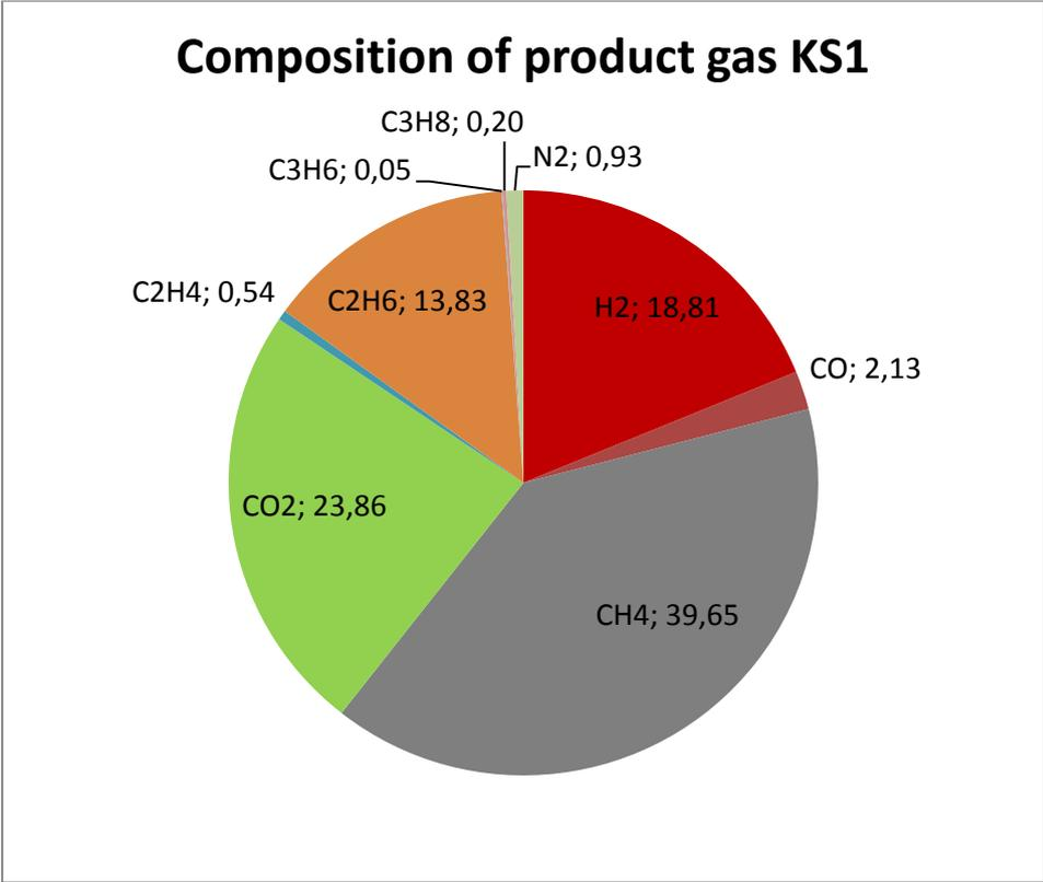
Figure 18: Composition of the product gas of experiment KS1.
