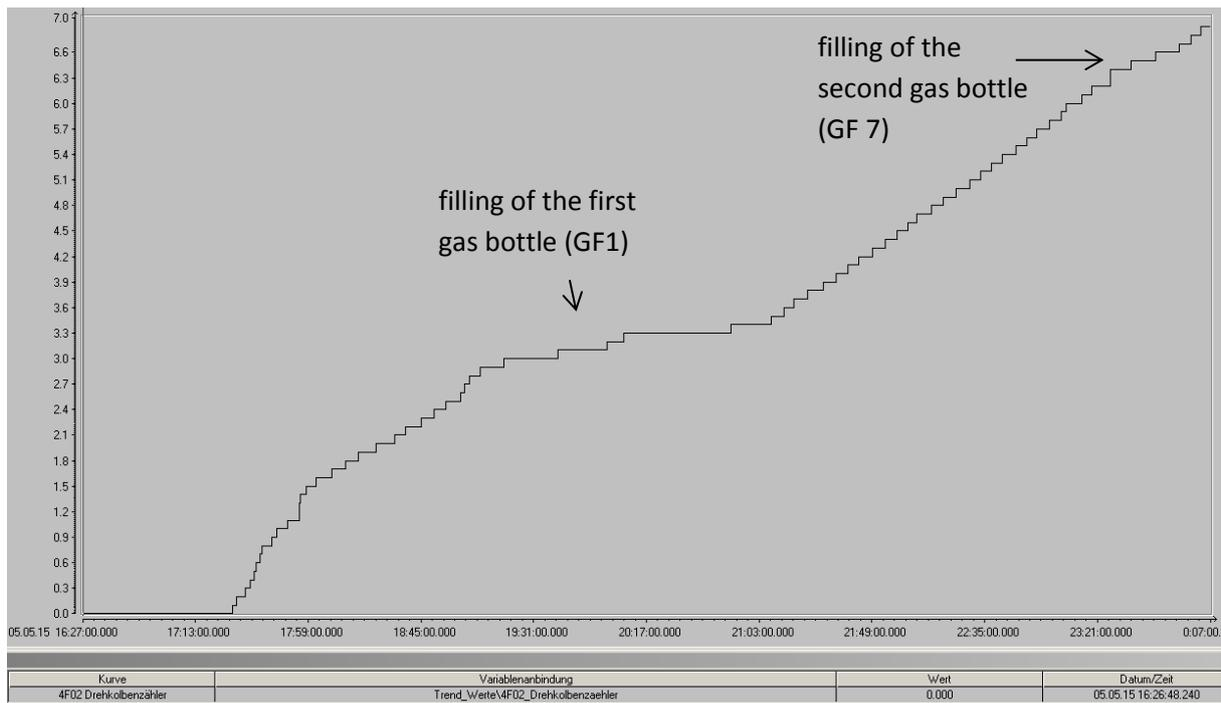
Figure 22: Amount of product gas in Nm<sup>3</sup>/h during steady state phase.
