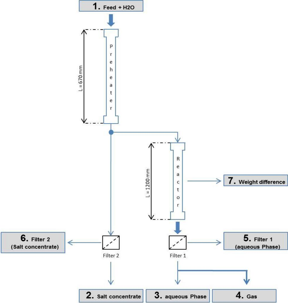
**Figure 4:** Schematic diagram of LENA
