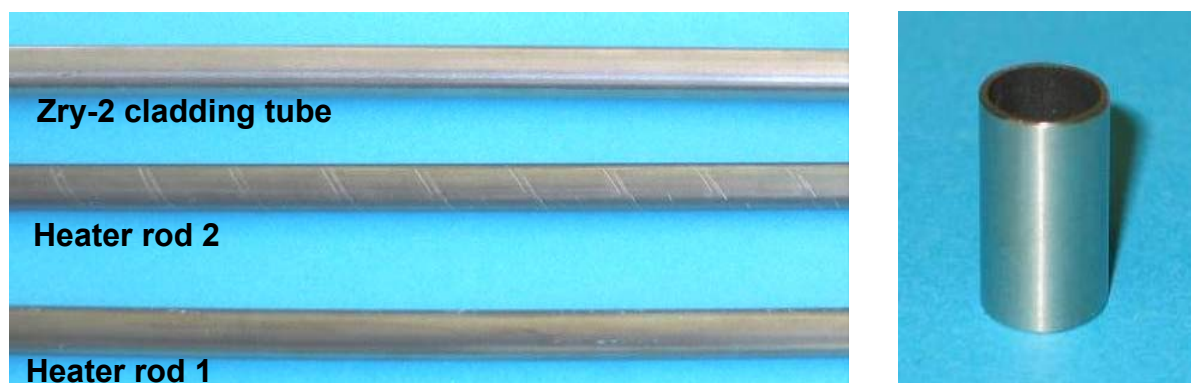
Fig. 2-2 Zircaloy-2 rod (top) and two prototype heaters as received (left) and sample for TG test (right)
