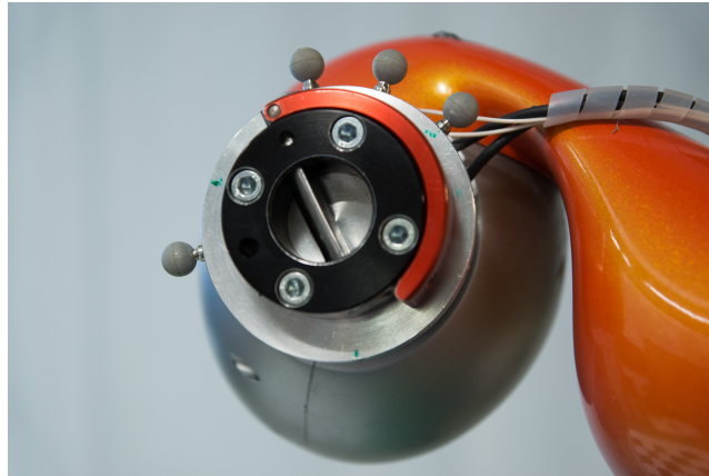
Figure 5.4.: The flange of a lightweight robot with markers on a rigid body.
