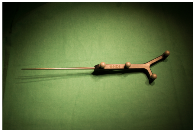
Figure 5.1.: The NDI pointer used in this work
