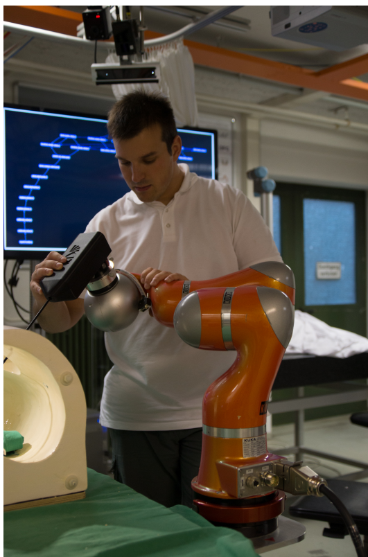
Figure 5.27.: An operator uses one of the robots in hands-on mode. In the top of the image parts of the perception system can be seen.
