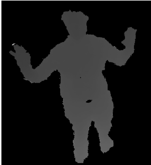
Figure 5.7.: The extracted depth image for a single human in a single depth frame from a Kinect™ 360 camera.
