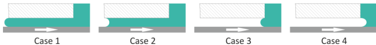
Figure 1.7: Schematic drawing of an upstream slot die section with the four stable pinning cases beneath the upstream lip. The white arrow marks the coating direction.
