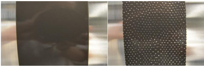
Figure 3.8: Stable LIB-electrode coating (left) and onset of film defects for a reduced film thickness (right) at the used experimental set-up.
