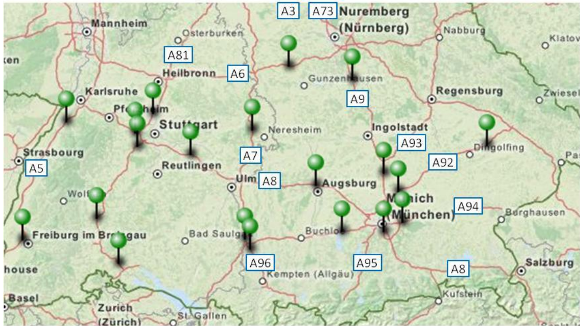
Figure 2: Allocation of fast charging stations in scenario 2 (150 km range, 20 charging stations placed)
