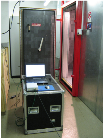
4.8.1: Alice's USRP2 transmitter with laptop (outside the chamber).
