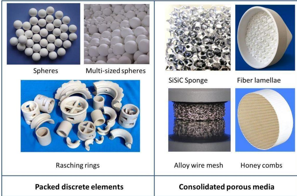
Figure 1.1: Some examples of commonly used porous inert media to support combustion; some pictures taken from [8]
