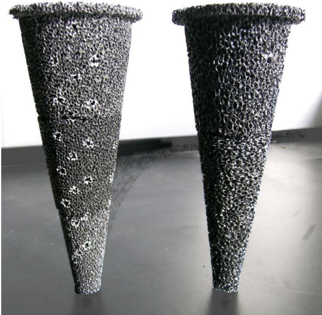
Figure 3.4: Photo of the used porous burners: left side 20 PPI, right side 10 PPI.
